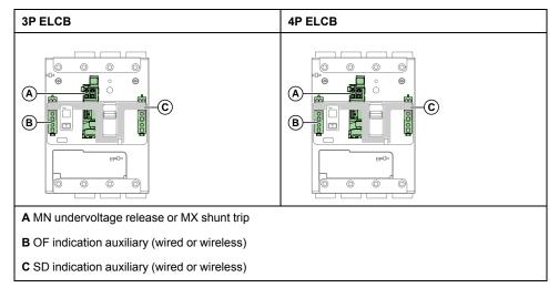
The following figures show the available slots for electrical auxiliary devices mounted outside the earth-leakage circuit breaker (ELCB). Two SDx modules can be installed.
