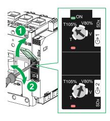
T SDT thermal fault indication T105% SDT thermal alarm: 105% Ir V80% SDV earth-leakage alarm: 80%  $I\Delta n$
