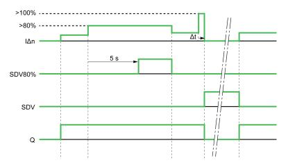
**IΔn** Earth-leakage current **SDV80%** Earth-leakage alarm
