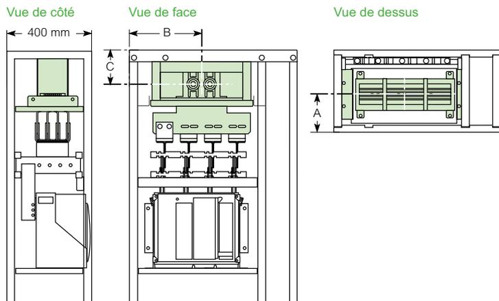
Circuit breaker NS/ MTZ1 3P-4P (fixed and withdrawable) - Depth: 800 mm
