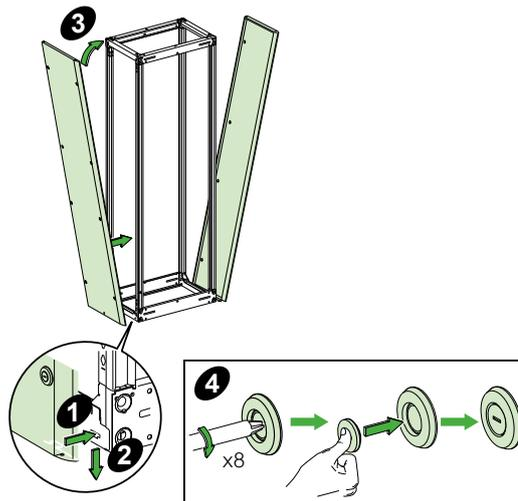
**Note:** panels equipped with a factory-fitted polyurethane (PUR) seal.
