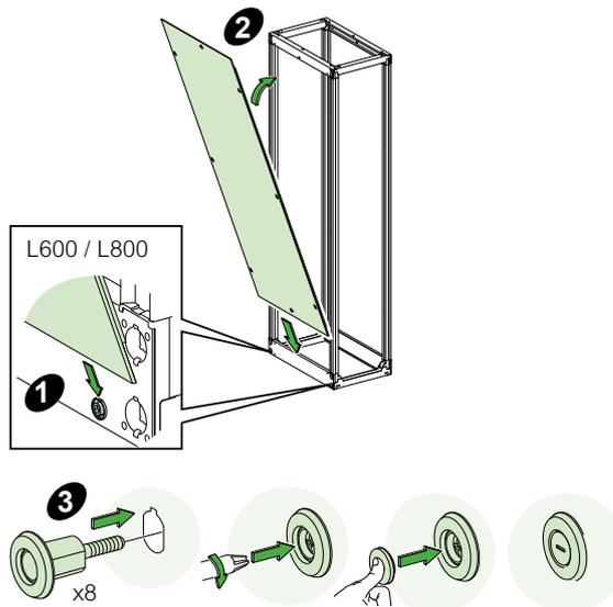
**Note:** panels equipped with a factory-fitted polyurethane (PUR) seal.
