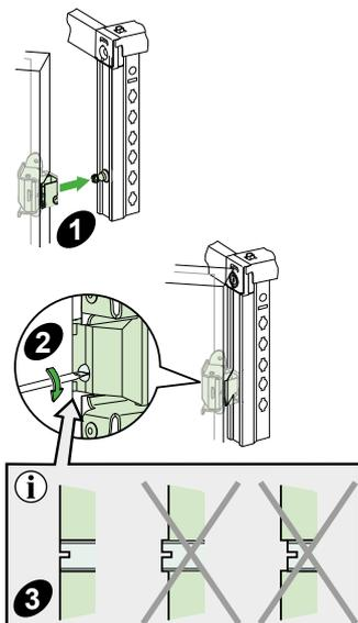
**Note:** the doors of switchboards protected to IP 55 are equipped with a factory-fitted polyurethane (PUR) seal.
