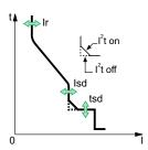
The short-time overcurrent pickup Isd sets the level of short-circuit current at which the circuit breaker trips when reaching the short-time overcurrent time delay.
