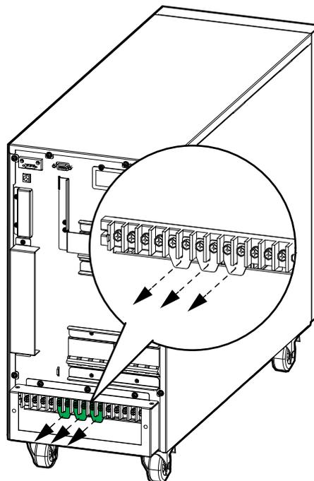
4. Route the power cables through the bottom of the conduit box.
