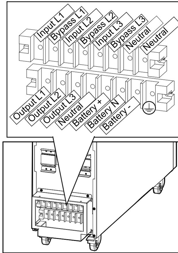
6. Connect the input, output, and bypass (if applicable) cables.
