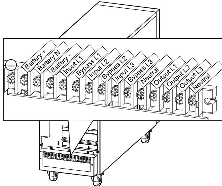
6. Connect the input, output, and bypass (if applicable) cables.
