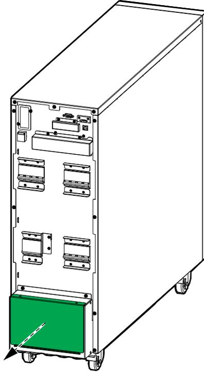
3. In dual mains systems, remove the three single mains brackets.
