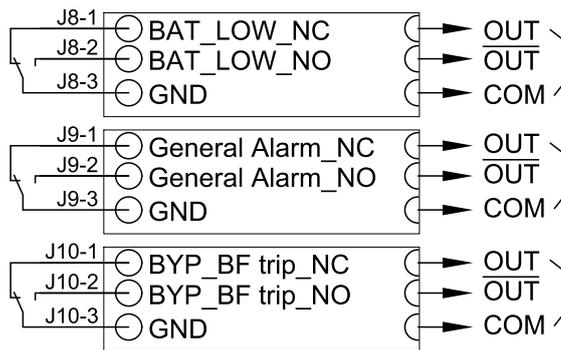
**Connect the Signal Cables in Parallel Systems**
