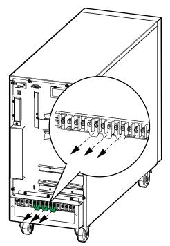
4. Route the power cables through the bottom of the conduit box.
