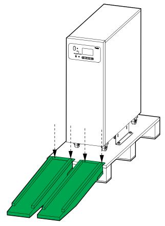
4. Loosen the bolts and remove the shipping brackets. Dispose of the shipping brackets.
