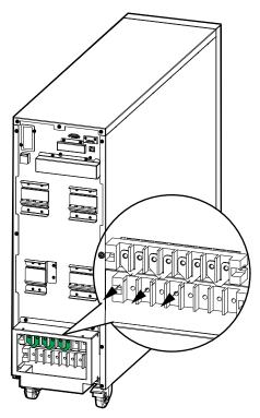
4. Route the power cables through the conduit box.
