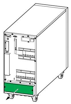
3. In dual mains systems, remove the three single mains brackets.
