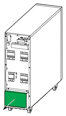
3. In dual mains systems, remove the three single mains brackets.
