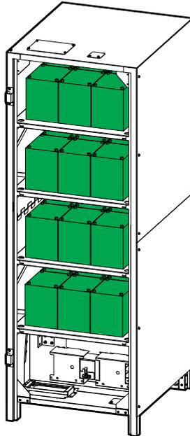
2. Connect the battery cables (Batt+, N, Batt-) from the batteries in the empty classic battery cabinet to the battery breaker.
