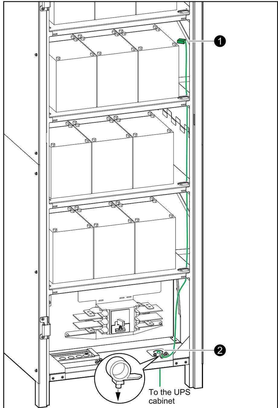
2. Route the battery temperature sensor cables through the top or the bottom of the empty classic battery cabinet to the UPS dry contact terminal J2-1 and J2-2 and connect as shown.
