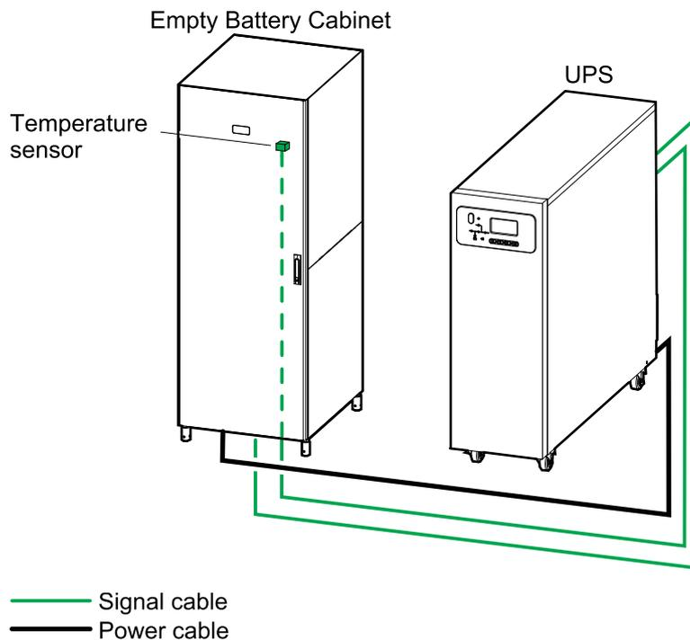
**NOTE:** The distance between the battery bank and the UPS must not exceed 200 m. Contact Schneider Electric for installations with a longer distance.
