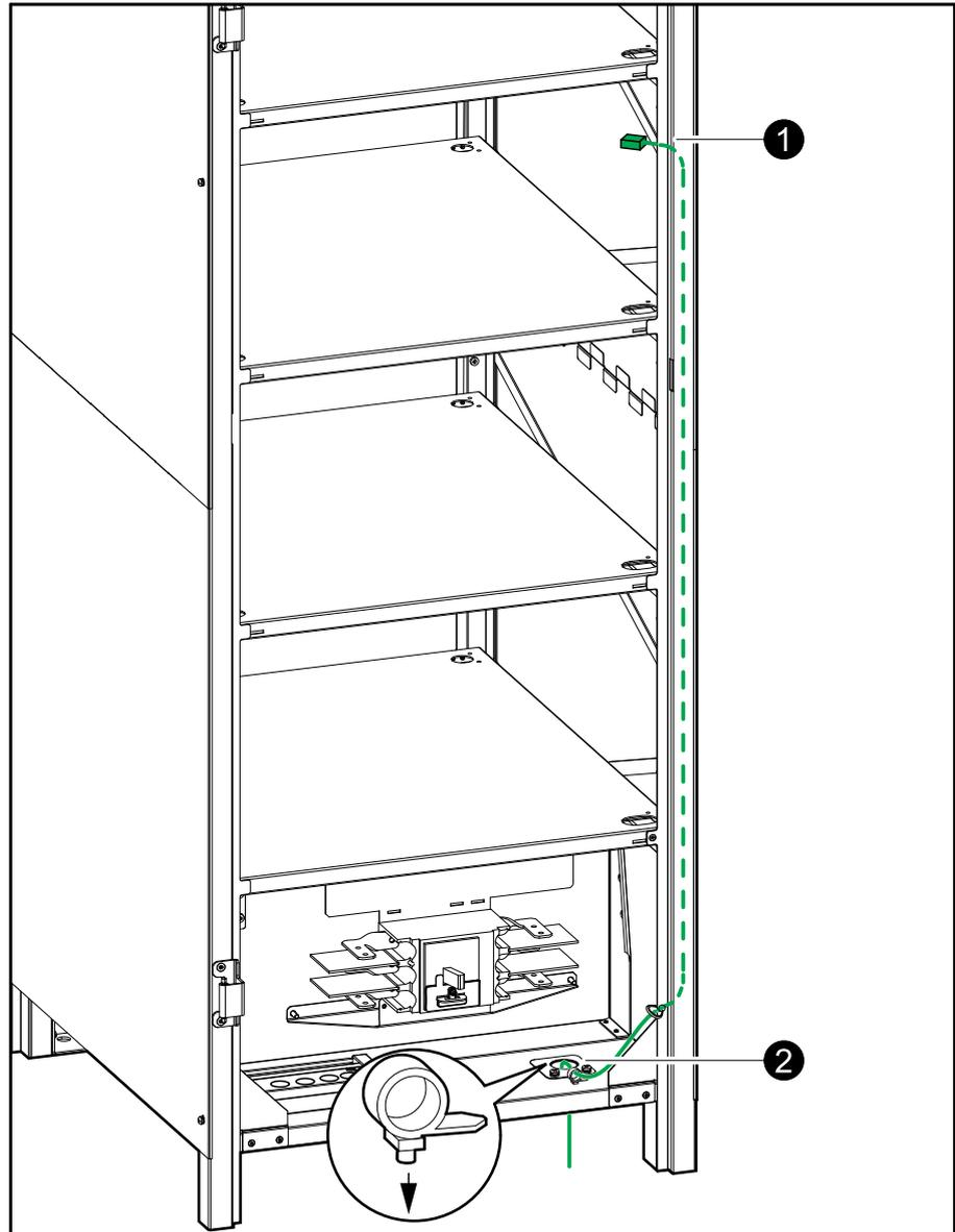
2. Route the battery temperature sensor cables through the top or the bottom of the empty battery cabinet to the UPS dry contact terminal J2-1 and J2-2 and connect as shown.
