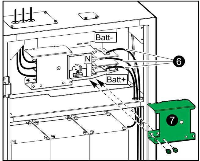
7. Install the protection cover over the terminals on the right side of the battery breaker.
