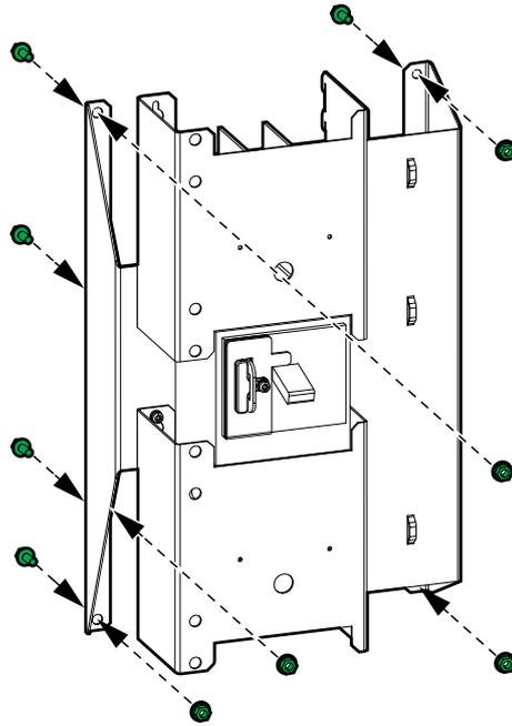
1. Measure and mark the holes for mounting the battery breaker kit in the metal box.
