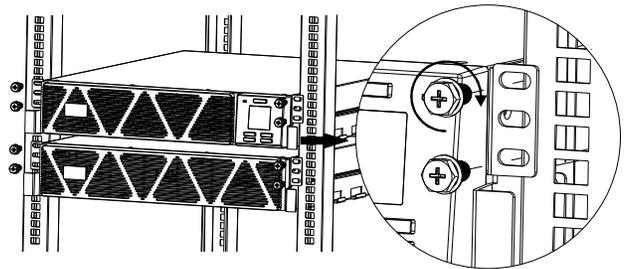
**NOTE:** Given the heavy weight, the use of rack-mount brackets is mandatory during rack installation (guide with L-shaped support). For the same reason, it is recommended that the UPS, battery pack be installed in the lower part of the rack cabinet. Optional rail kit accessory could be purchased separately if required.
