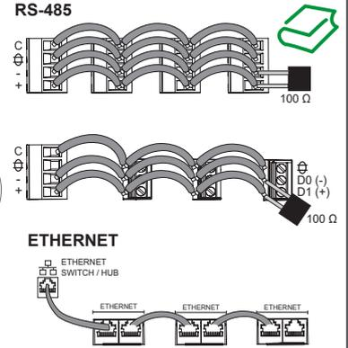
**en** Straight-line topology only. Loop or ring topology is not supported.
