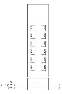
1 24 Vdc I/O power segment integrated into the bus bases
