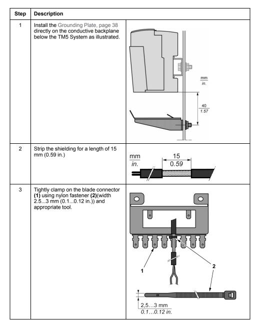
Alternative 2: Connect the shield of a cable via the grounding connector on the bus base of the TM5 I/O modules:
