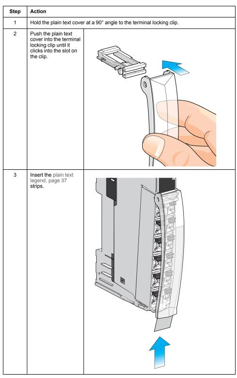
The covers are attached to the terminal locking clips:
