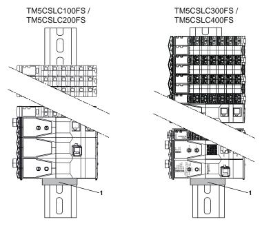
However, the TM5 Safety-Related System can also be mounted sideways on a vertical plane as shown below.
