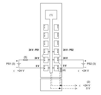
The following figure shows the wiring diagram for the TM5SPS2F:
