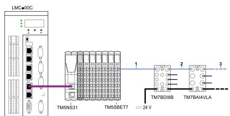
**1** Attachment IN cable: to connect a TM7 I/O block after a TM5 configuration using a TM5SBET7 transmitter module.
