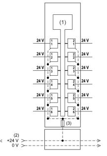
The following figure shows the wiring diagram for the TM5SPDD12F:
