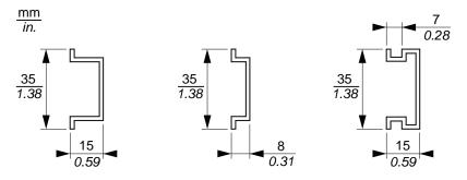
You can order a suitable DIN rail from Schneider Electric:
