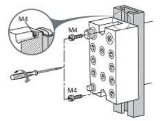
NOTE: Maximum torque to fasten the M4 screws is 0.6 N.m (5.3 lbf-in).
