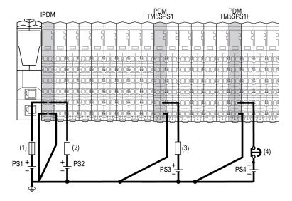
The following figure shows the wiring to supply the 24 Vdc I/O power segments:
