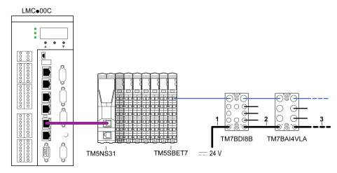
The following figure shows the power cables used in TM5/TM7 configurations:
