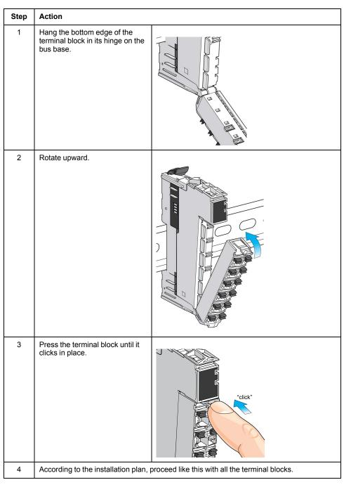
The following procedure describes how to mount the terminal block:
