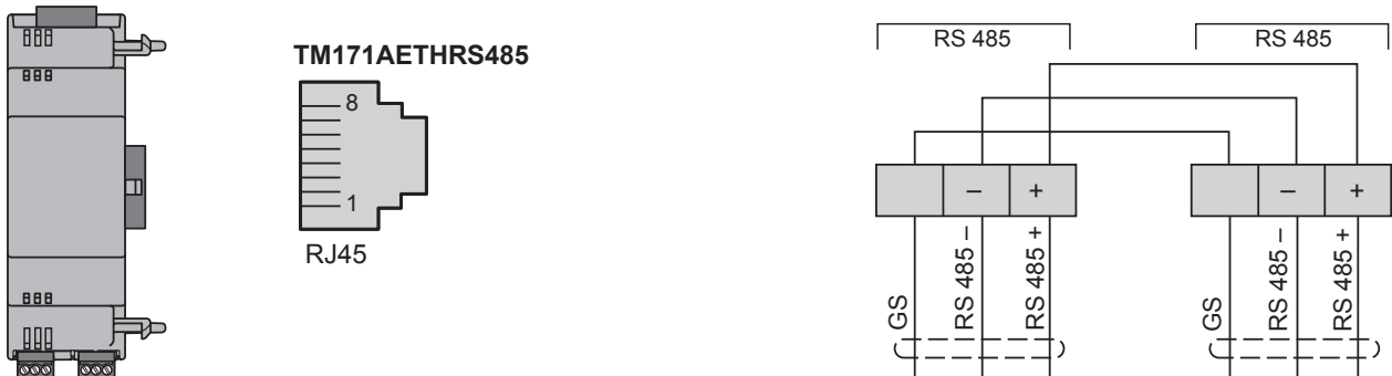
Fig. 37. ETHERNET, ETHERNET+RS485 Communication Modules
