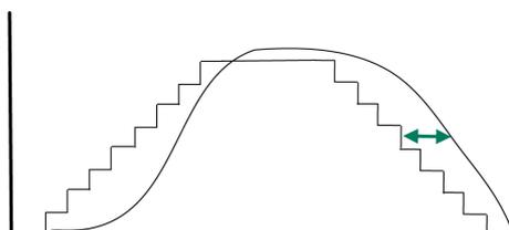
Increasing  $P8-27$  (GEARFILTT1) smooths the input command, but adds a delay.
