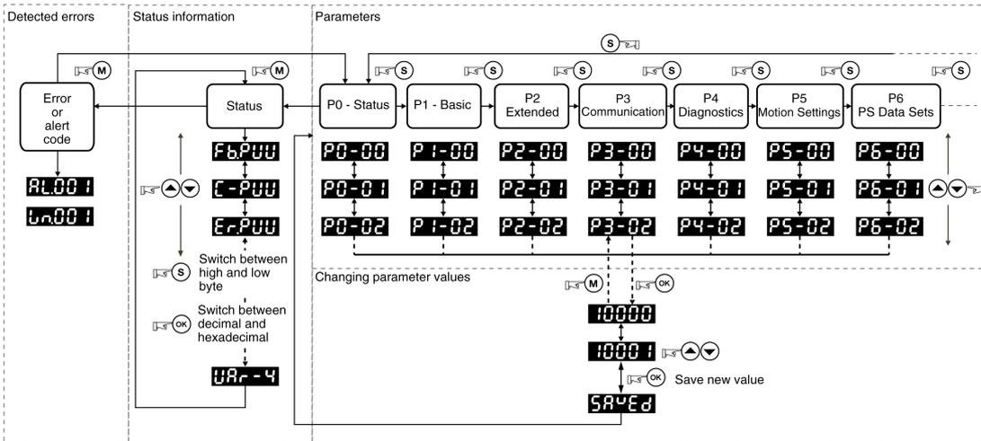
When the drive is powered on, the display shows the name of the selected status information function for approximately one second; after that, it displays the corresponding actual value or status value.
