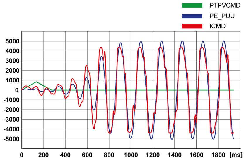
**NOTE:** The process of tuning requires trials of successive approximations. Values that are too high or too low relative to the other relevant values might cause instability. If it is necessary to have a low or high value of the parameter in the preceding example, you may need to adjust the values of the other relevant parameters to compensate and achieve a stable system.
