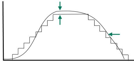
Increasing  $P8-28$  (GEARFILTT2) and  $P8-29$  (GEARFILTVELFF) compensate the delay, but adds overshoots.
