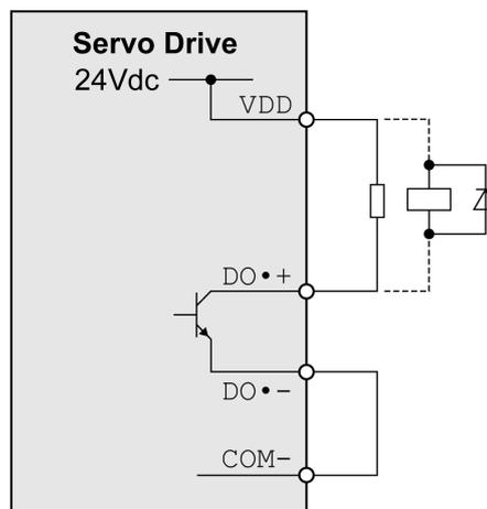
Example of digital outputs DO1 ... DO4 with external power supply (negative logic):
