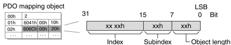
Subindex 00<sub>n</sub> of the communication object contains the number of valid subindex entries.
