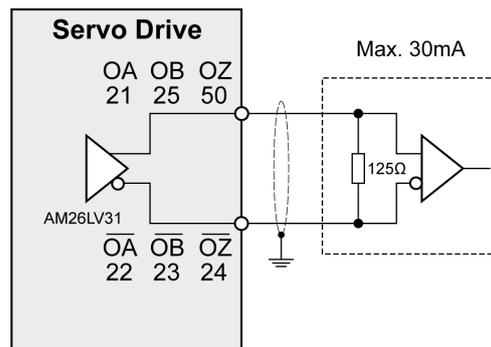
Example of encoder output signal, high-speed optocoupler.
