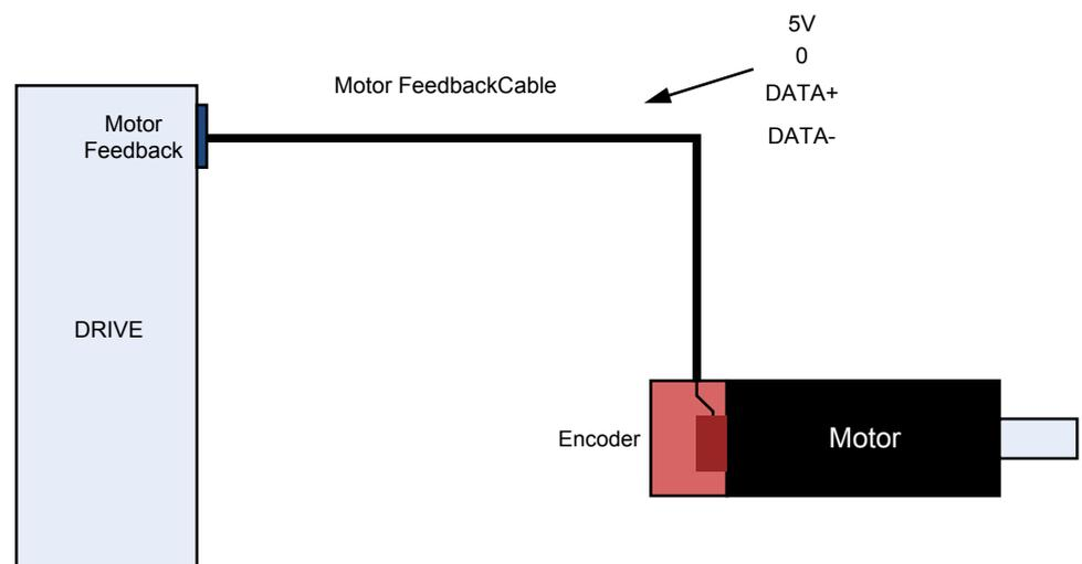
Single-turn encoder is connected to the servo drive over a motor feedback cable. The power to the encoder is supplied over the 5V output of the servo drive. As long as the servo drive is powered, the encoder is powered too, responding with an absolute position in a single revolution.
