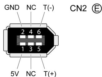
The motor encoder interface (CN2) is a 6-pin connector. The following table describes the contacts of the connector:
