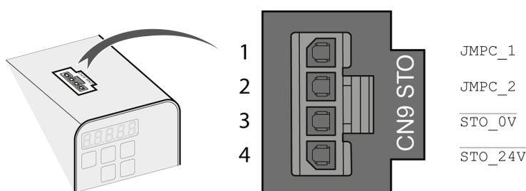
The STO interface (CN9) is a 4-pin female connector. The following table describes the contacts of the connector:
