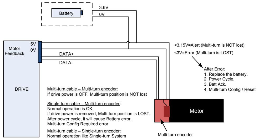
The multi-turn encoder is connected to the servo drive over a battery compartment, which is responsible to supply battery to the multi-turn subsystem in the encoder while power (5V) is off. The battery compartment contains circuitry which controls the switching between the power (5V) and the battery supply automatically.
