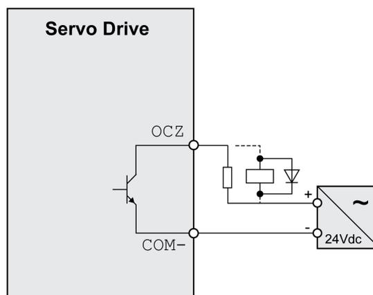
Inductive loads using DC voltages may damage the signal outputs. A protection circuit is required to protect the signal outputs against inductive loads.
