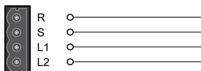
Wiring diagram logic supply LXM28E...M3X
