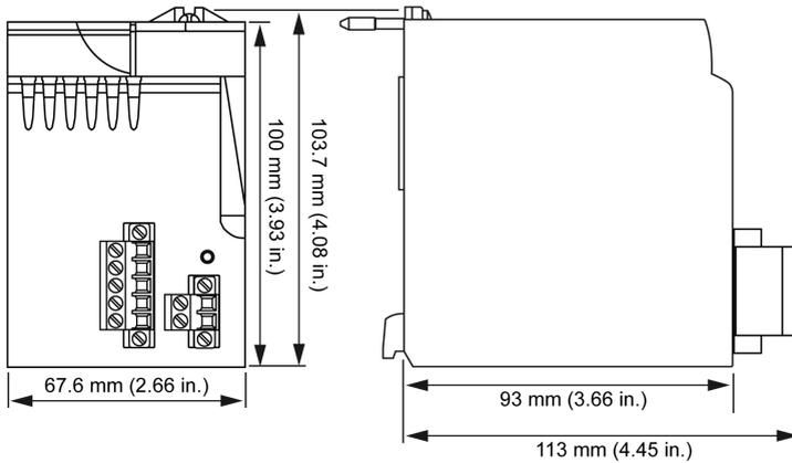
This figure shows the dimensions of a redundant power supply module:
