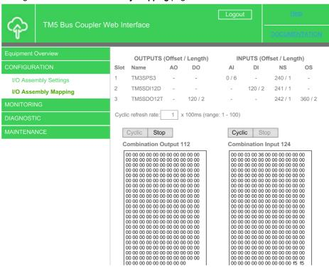
Below **OUTPUTS**, in the left part of the table, the composition of the combination output assembly (instance 112), which is made up of the data from the analog output (**AO** column) and digital output (**DO** column) assembly, and to the right, under **INPUTS** the combination input assembly (instance 124) with analog input (**AI** column), digital input (**DI** column), network status (**NS** column) and output status (**OS** column) are described.
