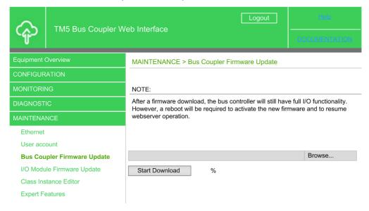
The Web server allows you to remotely monitor a TM5 EtherNet/IP Fieldbus Interface, to perform various maintenance activities, including modifications to data and configuration parameters, and change the state of the TM5 EtherNet/IP Fieldbus Interface. Ensure that the immediate physical environment of the machine and process is in a state that will not present safety risks to people or property before exercising control remotely.
