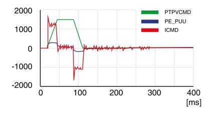
Example P8-03 (LTNP) value too high - oscillation at standstill (75 Hz)
