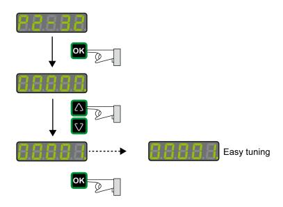
After you have started Easy Tuning via P2-32, the display of the HMI shows the progress as a percentage from tn000 to tn100.
