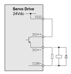
Example of digital outputs DO1 ... DO4 with external power supply (positive logic):
