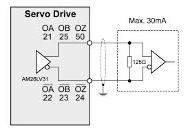
Example of encoder output signal, high-speed optocoupler.
