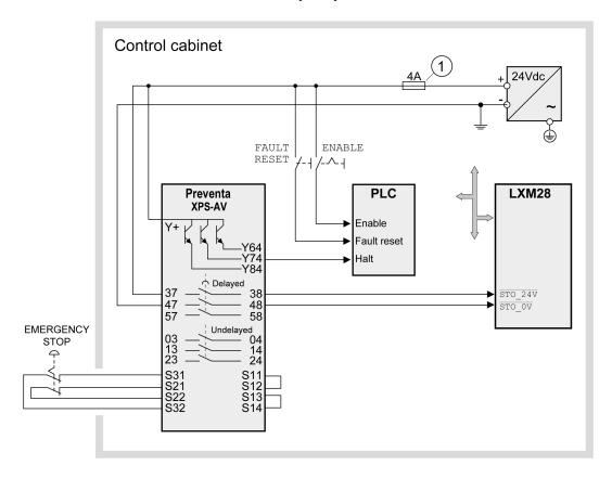
1 If the maximum output current of the 24 V power supply exceeds 4 A, a 4 A slow-blow fuse is required.
