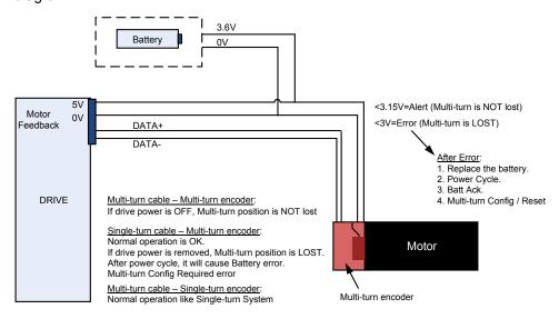
The multi-turn encoder is connected to the servo drive over a battery compartment, which is responsible to supply battery to the multi-turn subsystem in the encoder while power (5V) is off. The battery compartment contains circuitry which controls the switching between the power (5V) and the battery supply automatically.
