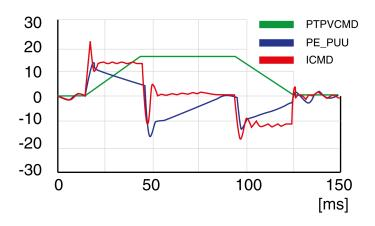
Example *P8-20* (NLPEAFF) minimum position deviation, short settling time, oscillation at standstill (120 Hz)
