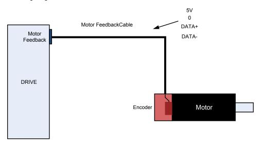
Single-turn encoder is connected to the servo drive over a motor feedback cable. The power to the encoder is supplied over the 5V output of the servo drive. As long as the servo drive is powered, the encoder is powered too, responding with an absolute position in a single revolution.
