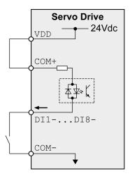
Example of digital input (negative logic) with external power supply:
