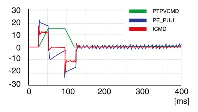
Example *P8-02* (LTNIV) position deviation decreases rapidly when target velocity is reached (90 Hz)
