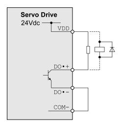
Example of digital outputs DO1  $\dots$  DO4 with external power supply (negative logic):
