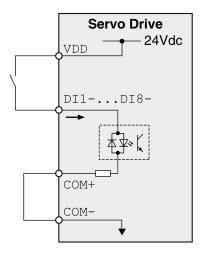
Example of digital input with external power supply (positive logic):
