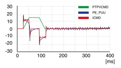
Example *P8-02* (LTNIV) value too high - oscillation at standstill, overshoot of position deviation (120 Hz)
