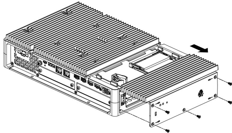
4. Insert the HDD or SSD into the slot.
