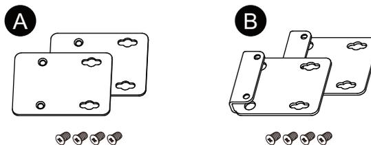
2. Remove the screws attached to the product (4 pieces), then use the screws for the book mount adapter to attach it to the product. When attaching to the top of the product, attach the B book mount adapter so that the protruding part faces the product.
