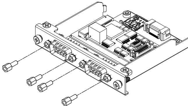
2. Disconnect the interface connector from the cartridge, and also disconnect the cable connected to the board.
