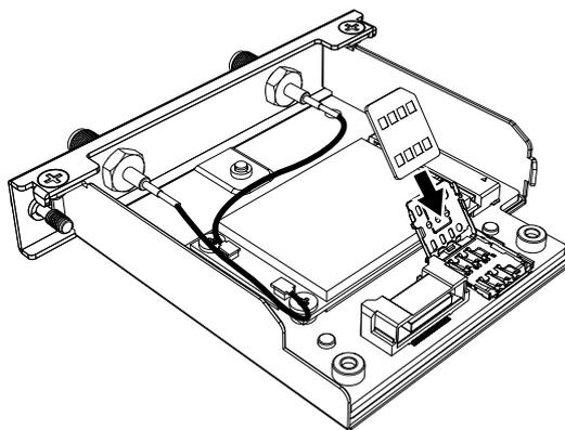
7. Close and slide the cover in the direction of the arrow to lock.
