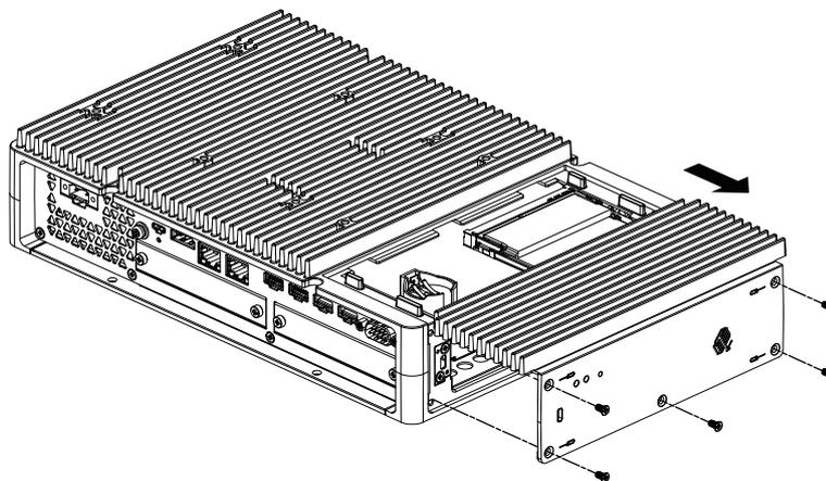
4. When equipped with M.2 SSD, remove the heat sink and heat sink pad (for top) before installing the FAN kit. For information on the heat sink and heat sink pad for M.2 SSD, see M.2 SSD Installation, page 96.
