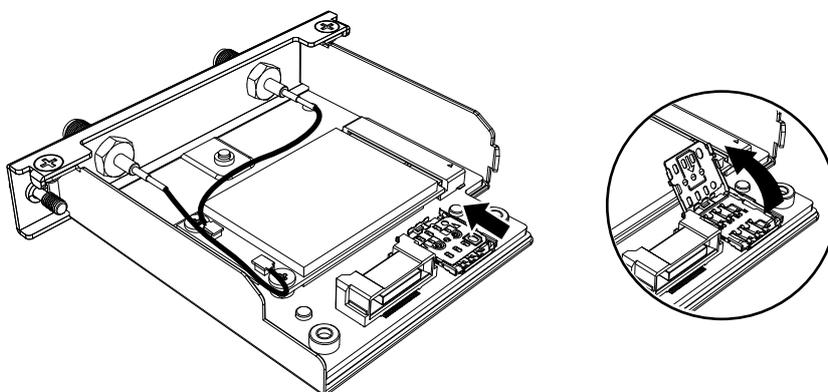
6. Insert the SIM card into the slot.
