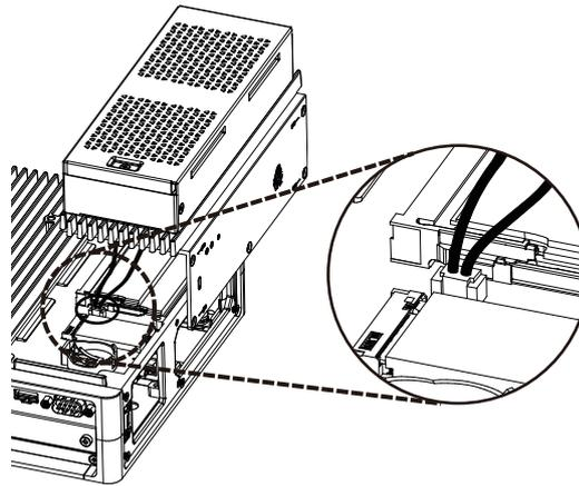
6. Using the screws removed in step 3, secure the FAN kit.
