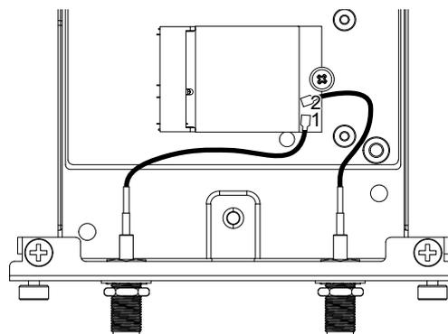
5. Attach this interface to the product. Attach the antenna only after mounting the product on the panel.
