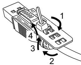
4. While pressing the grip on the clip, insert the cable from step 3 all the way into the USB host interface. Make sure that the tab of the clip is secured to the USB cable attached to this product.
