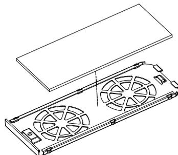
6. Re-insert the fan filter tray and tighten the screw.
