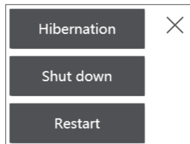
**NOTE:** With HORM enabled, using the Hibernation icon to hibernate the operating system will overwrite the previously saved state in HORM with the current system state. When you reboot the system, the system starts up in the state saved at hibernation. After that, even with HORM enabled if the power is shut off, the system returns to the state saved at hibernation.
