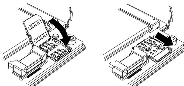
**NOTE:** When removing, inserting, or replacing the SIM card, 4G Cellular must be reset to its factory default. From 4G Cellular Settings, page 135, perform step 1.
