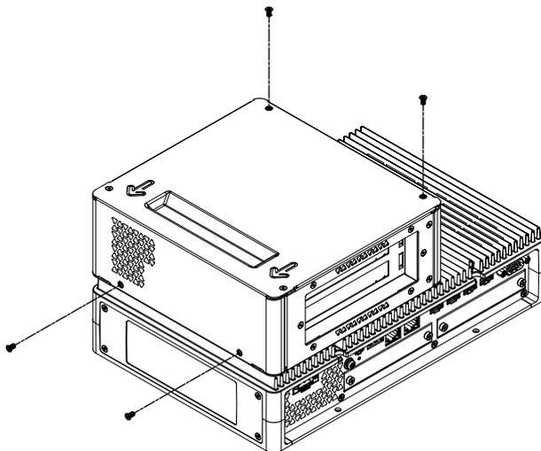
4. Slide the cover in the direction of the arrow on the top of the cover, and remove it.
