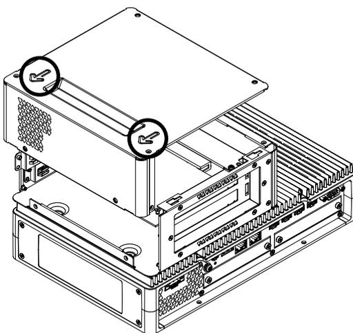
5. Remove the screw from the interface cover, then remove the cover.
