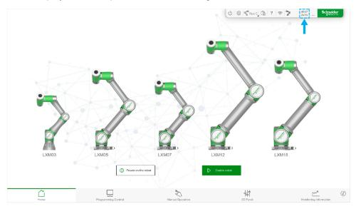
The checksum is used to represent the configuration of the safety-related parameters of the Lexium Cobot in the form of letters and numbers. If the safety-related parameters are changed, the checksum changes accordingly.
