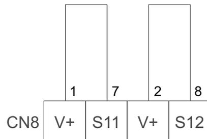
The following figure presents the wiring of an external emergency stop.
