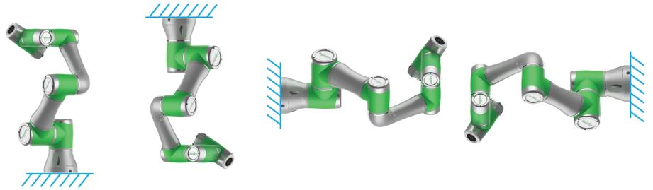
In case the Lexium Cobot Arm is mounted on a moving platform (for example, linear axis or moving platform), high acceleration of the moving ground base might be interpreted by the Lexium Cobot Arm as a collision.
