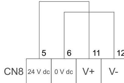
The following figure presents the wiring of the external power supply.
