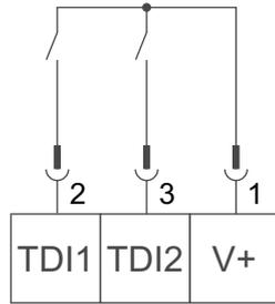
The following figure presents the source wiring of the controller digital inputs. Sink or source can be configured on the digital input settings by the application.
