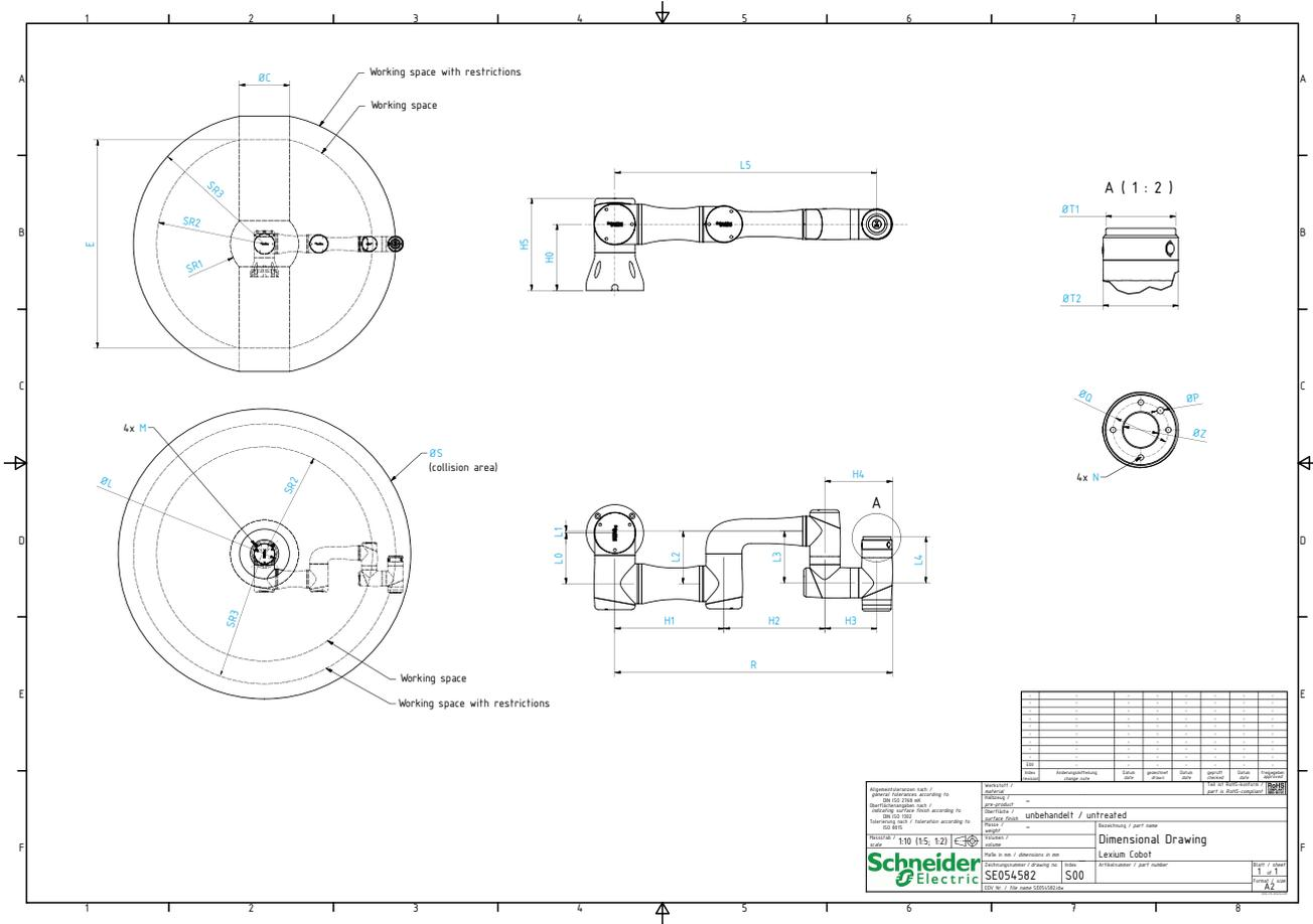
The possible working space of the Lexium Cobot Arm is represented as a flattened sphere. The flattenings exist above and below the Lexium Cobot Arm within a cylinder of 226 mm (8.9 in) diameter around the base (joint 1).
