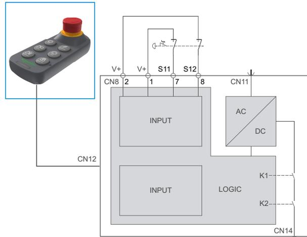
The Lexium Cobot Controller can also control other systems with the following safety-related outputs:
