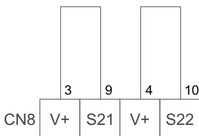
The following figure presents the default wiring of an external protective stop device.
