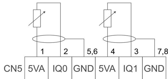
The following figure presents the wiring of the analog outputs at the Lexium Cobot Controller (CN5).
