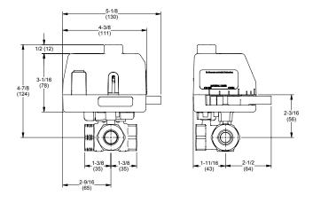
An additional 1 inch is required to remove the actuator from the valve.
