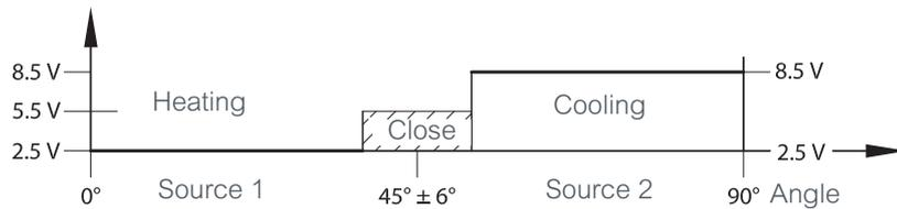
Heating connected to port 1 and 4
