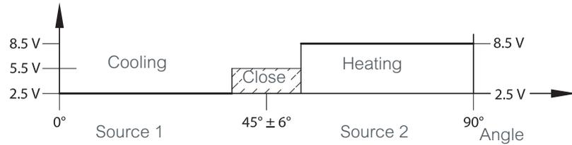
Cooling connected to port 1 and 4
