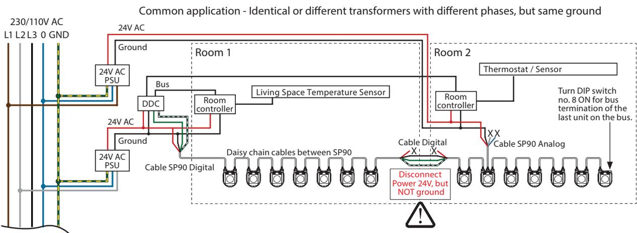
Wires that ends in an "X" must be properly terminated.
