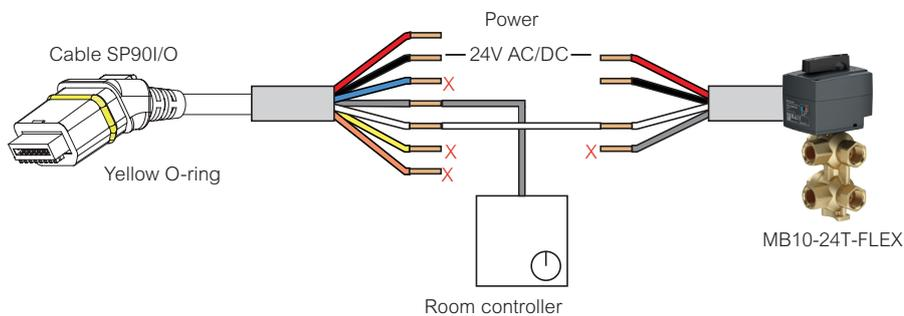
In this wiring example the feedback of position alarms from the MB10 is sacrificed for the use of a room controller or thermostat with 0-10V signal.
