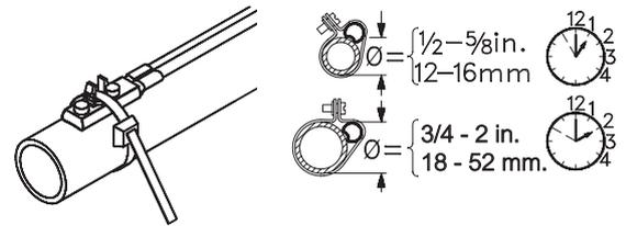
Cable ties of between 4.5mm and 5mm width will fit between the spring forks.
