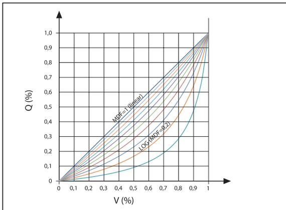
This Alpha Curve adjustment allows the SP90 to adapt to a specific model of heat exchanger curve to ensure a linear response of heat emission according to the valve position/ flow rate.
