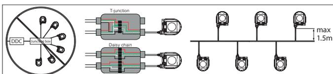
If the supply voltage to the first device in the daisy chain is lower than 24V AC/DC, or long thin cables other than SP90 cables are
