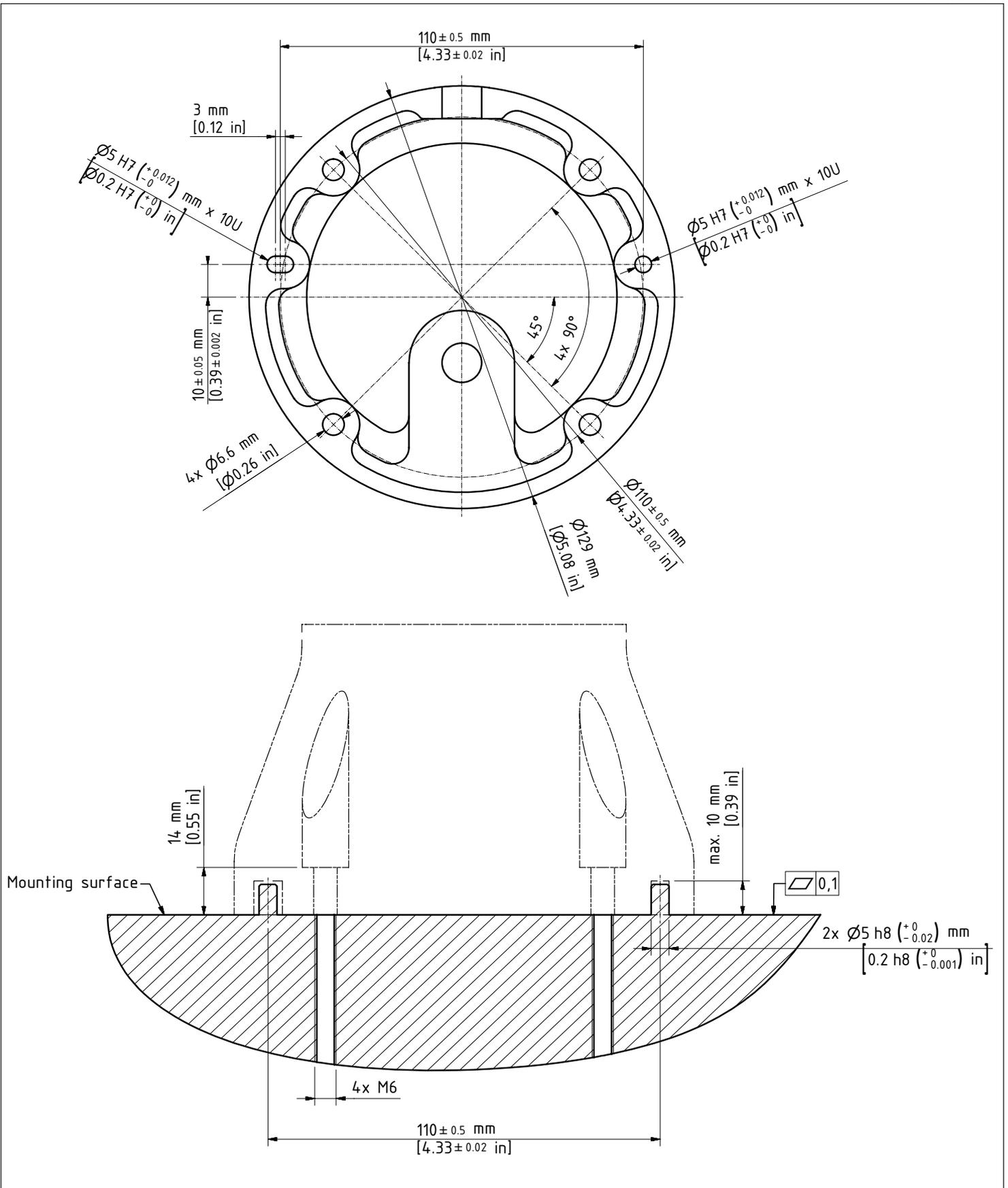
**en** The Lexium™ Cobot Controller is intended to be placed on a plane surface. Ensure that a clearance of 100 mm (3.9 in) is respected on each side of the Lexium™ Cobot Controller for sufficient airflow.
