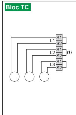
(1) : - It is essential that jumpers remain in position when metering device is not connected.
