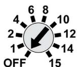
The SDTAM thermal fault module incorporates an auto-reset delay setting dial.
