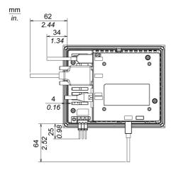
**NOTE:** All the above values are designed with cable bending in mind. The dimensions given here are representative values depending on the type of connection cable in use. Therefore, these values are intended for reference only.
