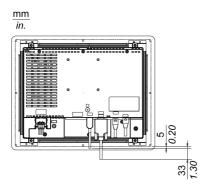
**NOTE:** All the above values are designed with cable bending in mind. The dimensions given here are representative values depending on the type of connection cable in use. Therefore, these values are intended for reference only.
