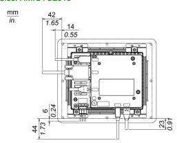
**NOTE:** All the above values are designed with cable bending in mind. The dimensions given here are representative values depending on the type of connection cable in use. Therefore, these values are intended for reference only.
