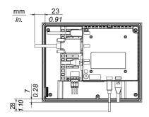
**NOTE:** All the above values are designed with cable bending in mind. The dimensions given here are representative values depending on the type of connection cable in use. Therefore, these values are intended for reference only.
