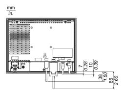
**NOTE:** All the above values are designed with cable bending in mind. The dimensions given here are representative values depending on the type of connection cable in use. Therefore, these values are intended for reference only.
