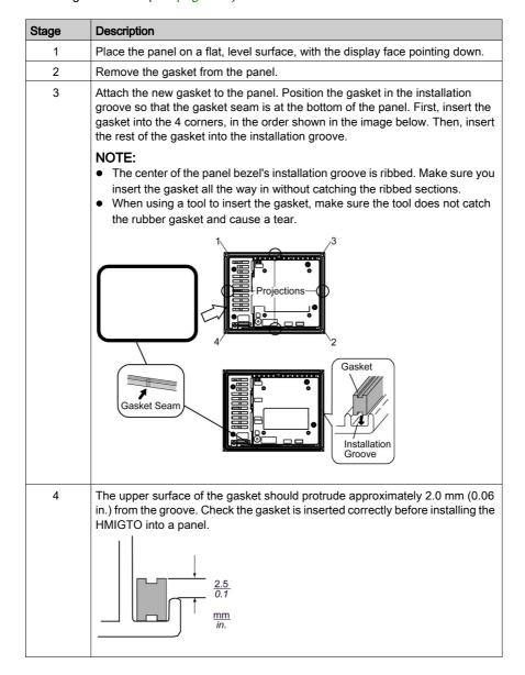
The gasket must be inserted correctly into the groove for IP65f moisture resistance for the panel (IP66k moisture resistance for HMIGTO2315/HMIGTO5315/HMIGTO6315.
