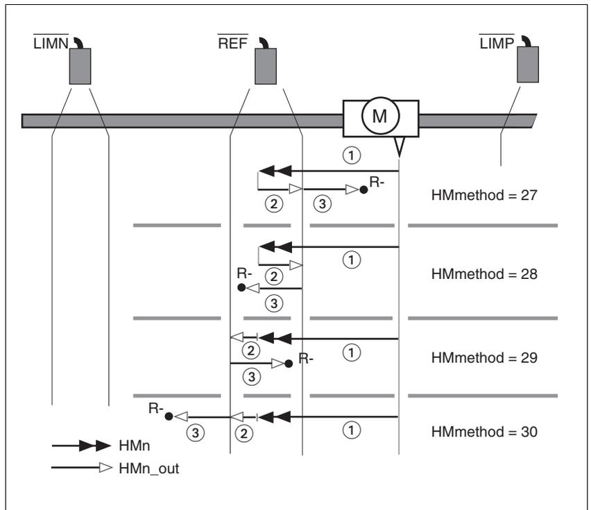
Figure 8.7 Reference movements to the reference switch
