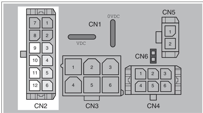
Figure 6.9 Pin assignment printed circuit board connector
