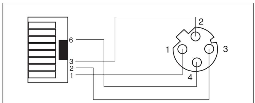
Figure 6.11 Pin assignment RJ45 to M12
