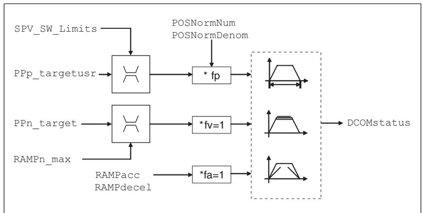
Figure 8.4 Operating mode Profile Position, effect of adjustable parameters
