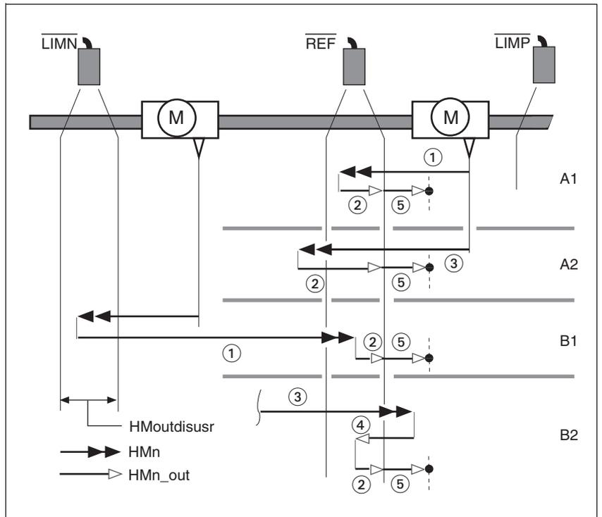
Figure 8.11 Reference movements to the reference switch
