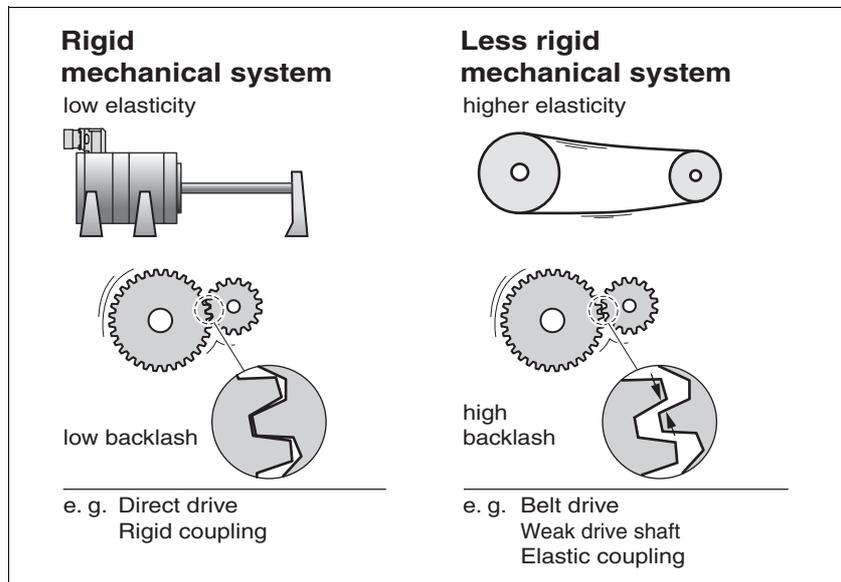
Figure 7.24 Rigid and less rigid mechanical systems
