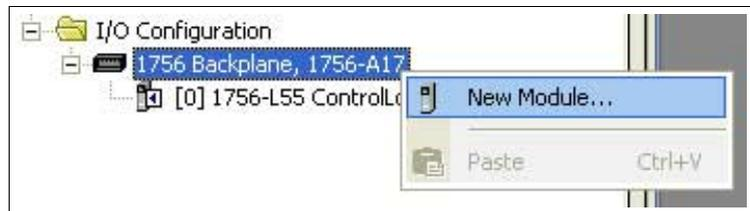
Figure 7.8 RSLogix 5000 - "New Module"
