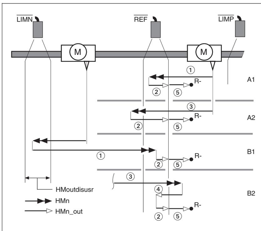
Figure 8.8 Reference movements to the reference switch
