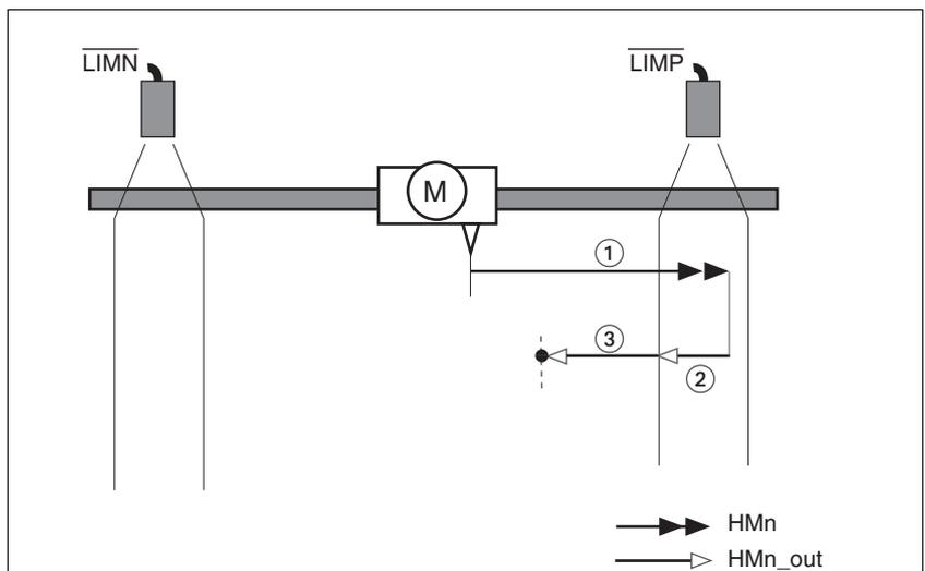
Figure 8.9 Reference movement to the positive limit switch
