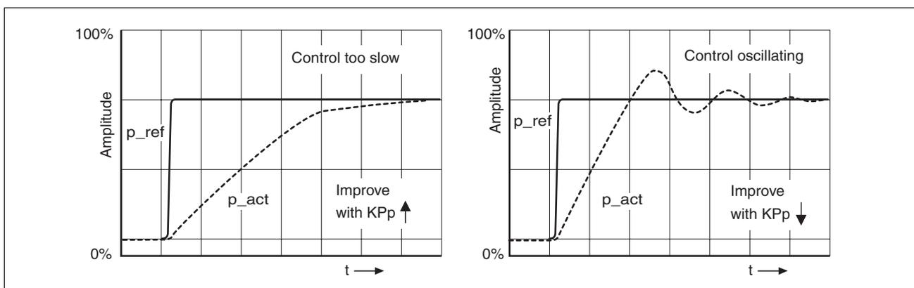
Figure 7.29 Optimizing inadequate position controller settings
