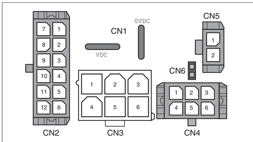
Figure 3.3 Overview of printed circuit board connectors
