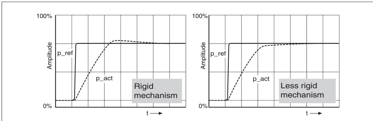
Figure 7.28 Step responses of a position controller with good control performance
