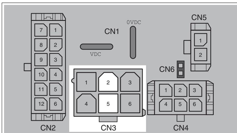
Figure 6.12 Pin assignment printed circuit board connector
