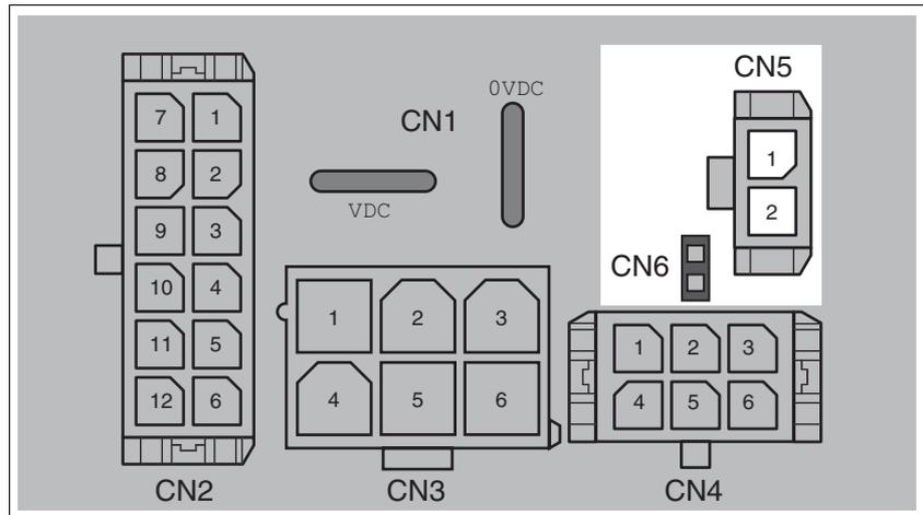
Figure 6.14 Pin assignment of safety function
