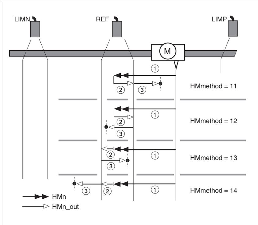
Figure 8.10 Reference movements to the reference switch
