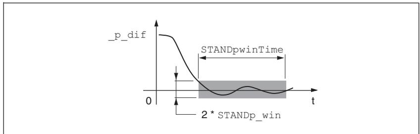
Figure 8.23 Standstill window
