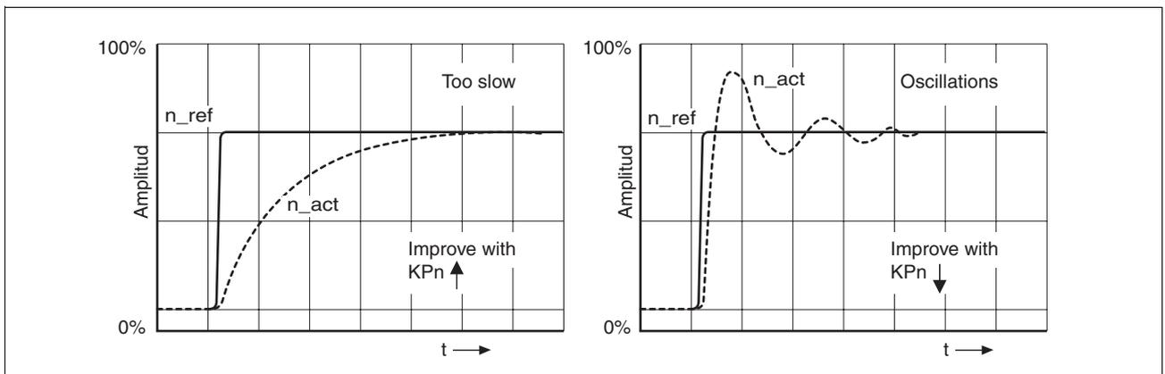
Figure 7.27 Optimizing inadequate velocity controller settings
