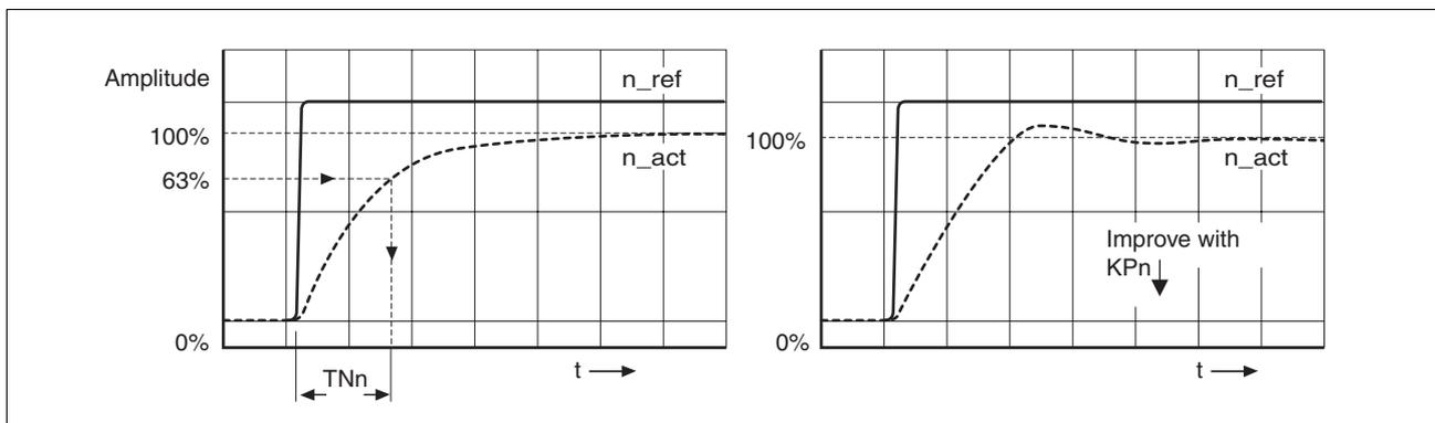
Figure 7.25 Determining "TNn" for the aperiodic limit
