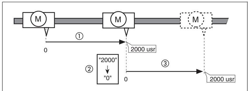
Figure 8.13 Positioning by 4000 usr units with position setting
