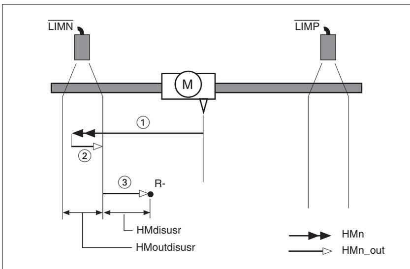
Figure 8.6 Reference movement to the negative limit switch
