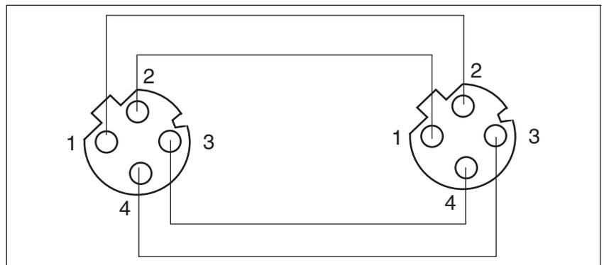
Figure 6.10 Pin assignment M12 to M12
