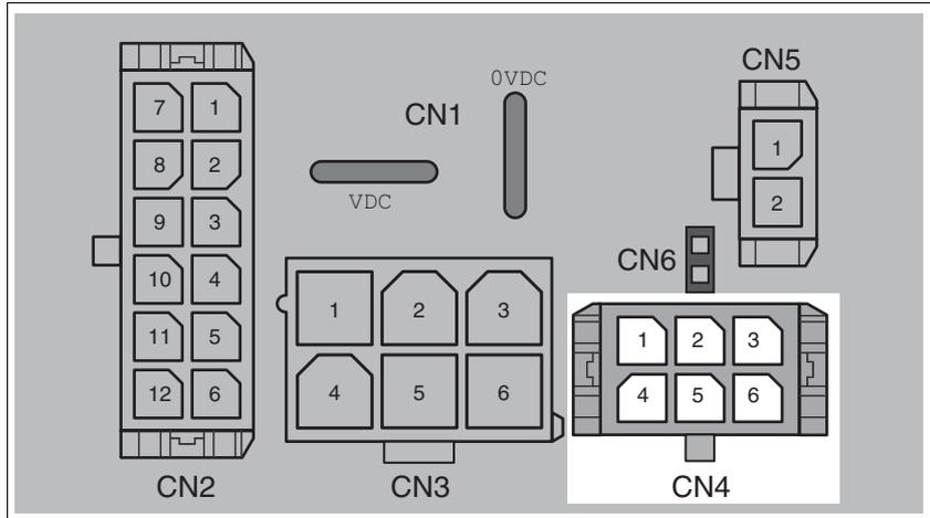
Figure 6.13 Pin assignment printed circuit board connector
