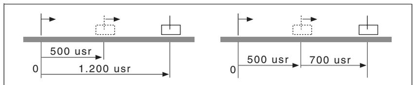
Figure 8.3 Absolute positioning (left) and relative positioning (right) Absolute positioning (left) and relative positioning (right)
