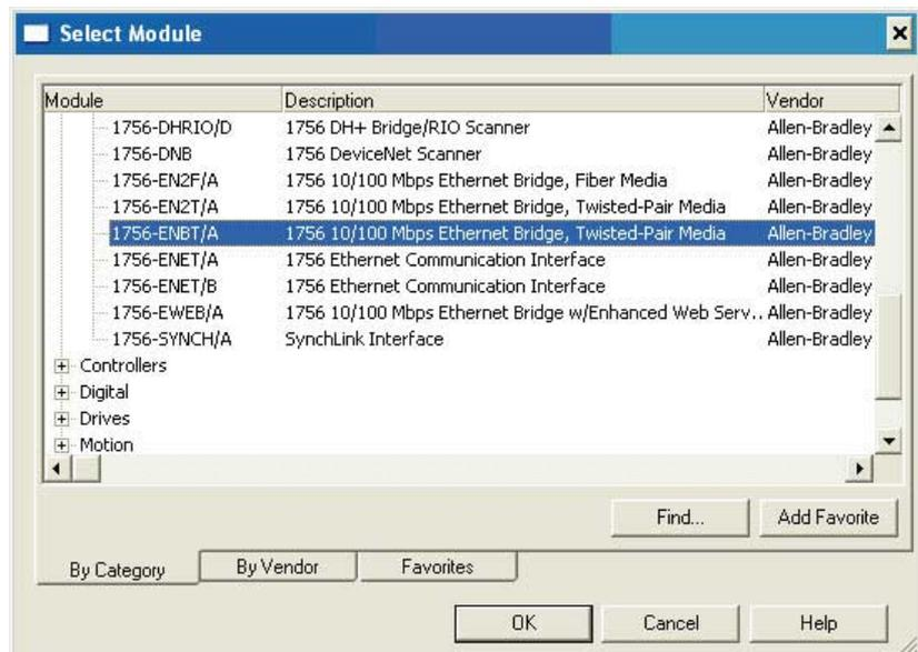
Figure 7.10 RSLogix 5000 - "Ethernet Bridge"
