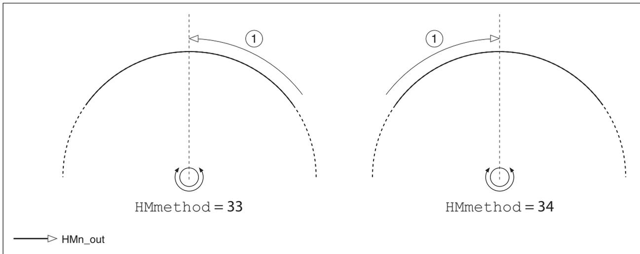
Figure 8.12 Reference movements to the index pulse
