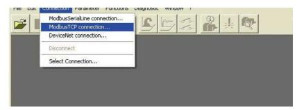
Figure 7.2 Selecting a Modbus TCP connection
