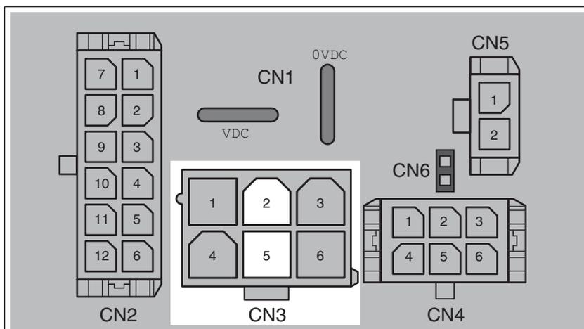
Figure 6.10 Pin assignment printed circuit board connector
