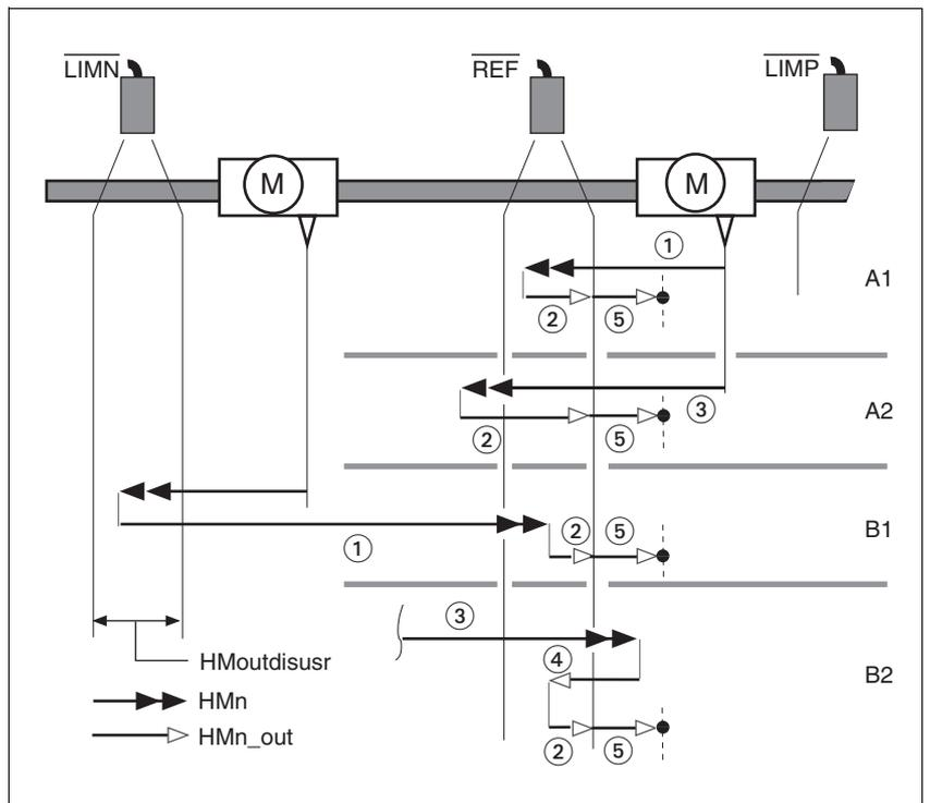
Figure 8.21 Reference movements to the reference switch
