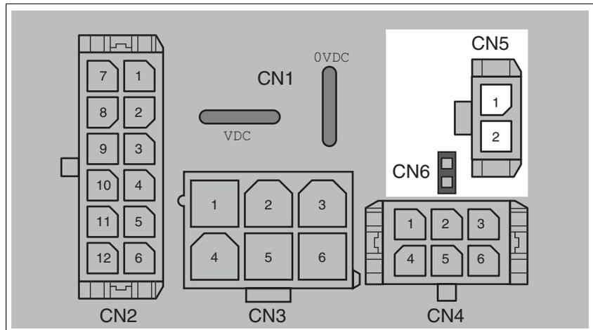
Figure 6.12 Pin assignment of safety function
