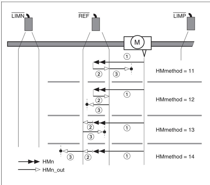
Figure 8.20 Reference movements to the reference switch
