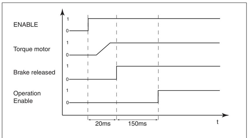
Figure 8.34 Releasing the holding brake
