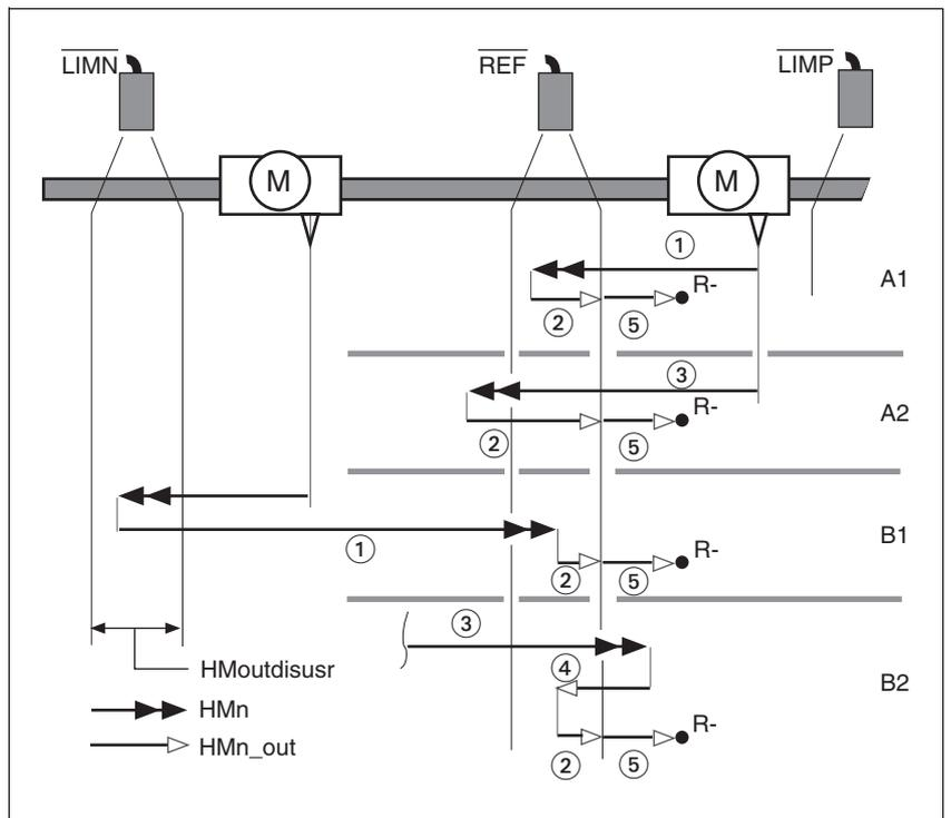
Figure 8.18 Reference movements to the reference switch
