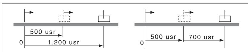
Figure 8.10 Absolute positioning (left) and relative positioning (right)
