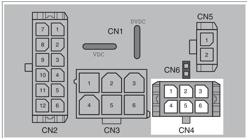
Figure 6.11 Pin assignment printed circuit board connector
