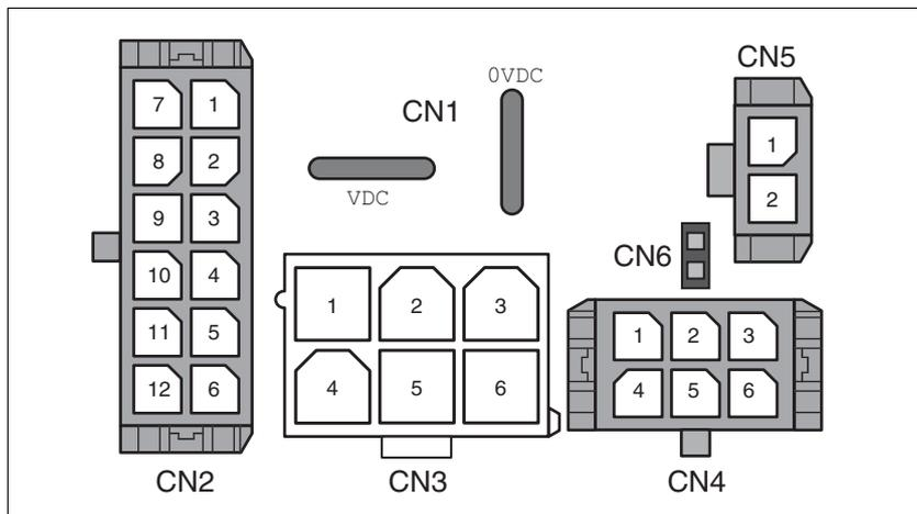
Figure 3.3 Overview of printed circuit board connectors
