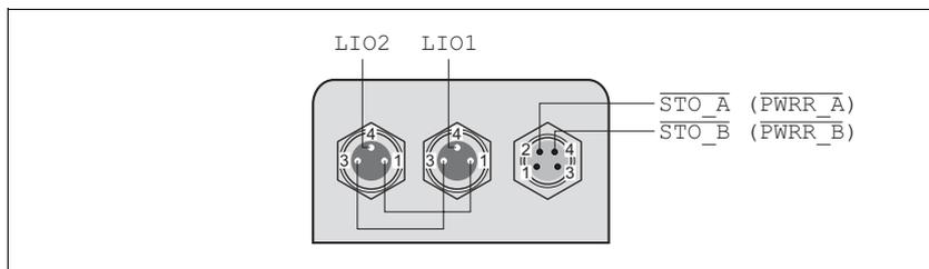
Figure 6.14 Pin assignment
