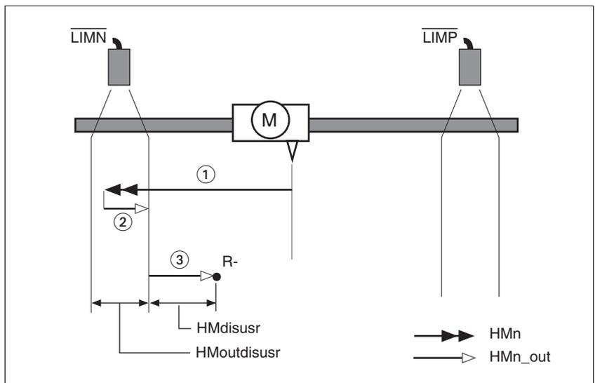
Figure 8.16 Reference movement to the negative limit switch
