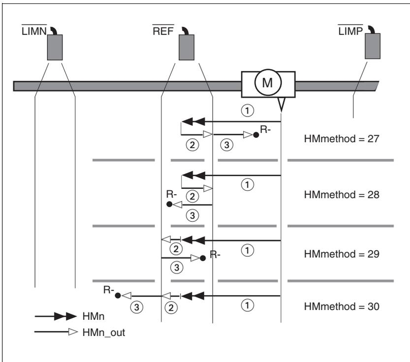
Figure 8.17 Reference movements to the reference switch
