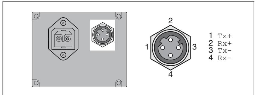
Figure 6.9 Pin assignment industrial connector
