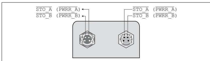
Figure 6.15 Pin assignment
