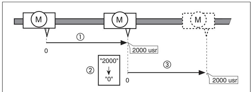
Figure 8.23 Positioning by 4000 usr units with position setting
