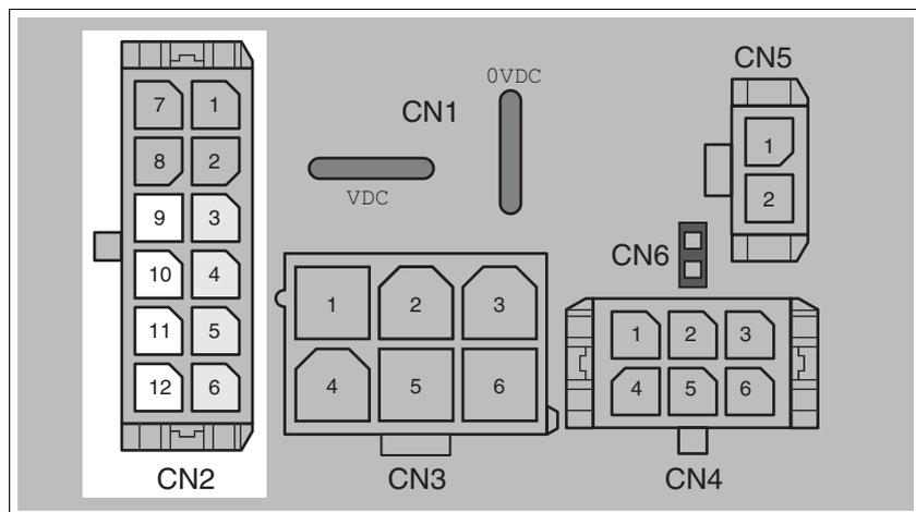
Figure 6.8 Pin assignment printed circuit board connector
