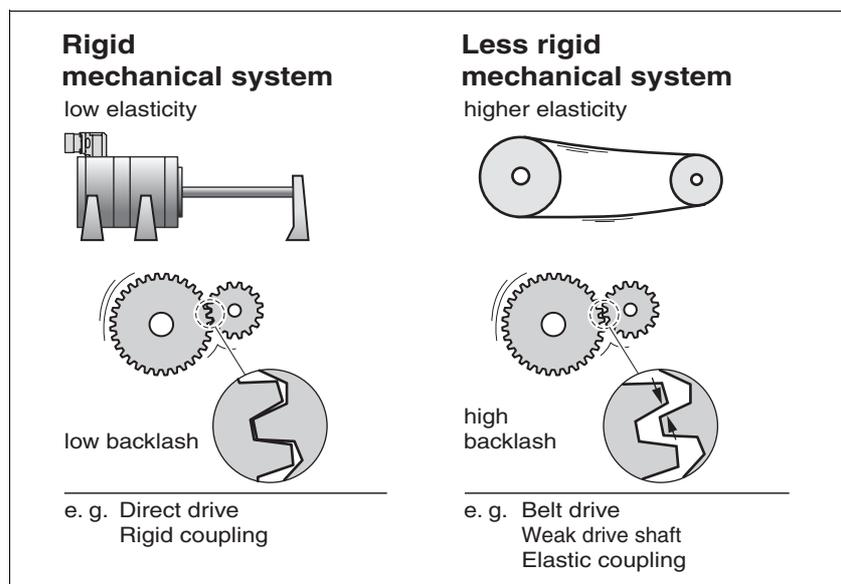
Figure 7.8 Rigid and less rigid mechanical systems
