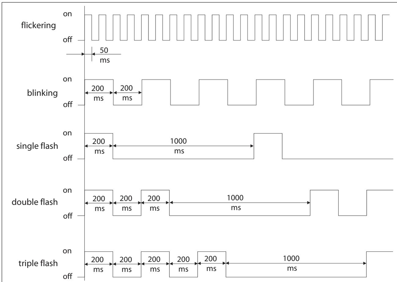
Figure 10.1 LED signals (selection)
