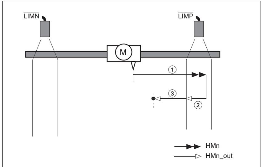
Figure 8.19 Reference movement to the positive limit switch
