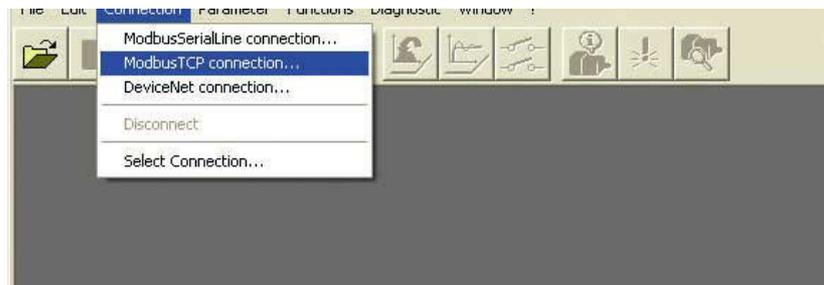
Figure 7.2 Lexium CT, Selecting a Modbus TCP connection
