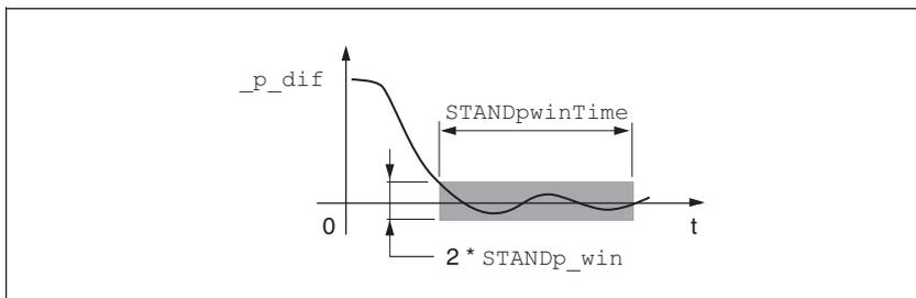
Figure 8.33 Standstill window
