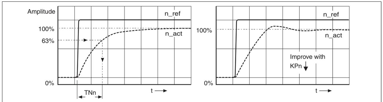
Figure 7.9 Determining "TNn" for the aperiodic limit
