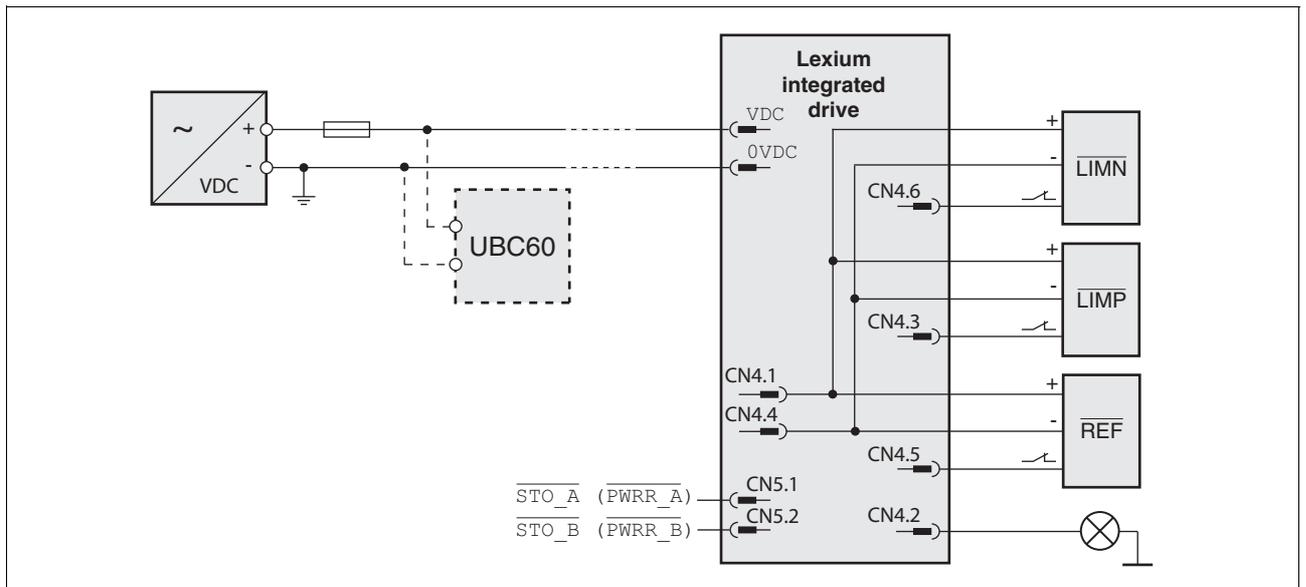
Figure 9.1 Wiring example
