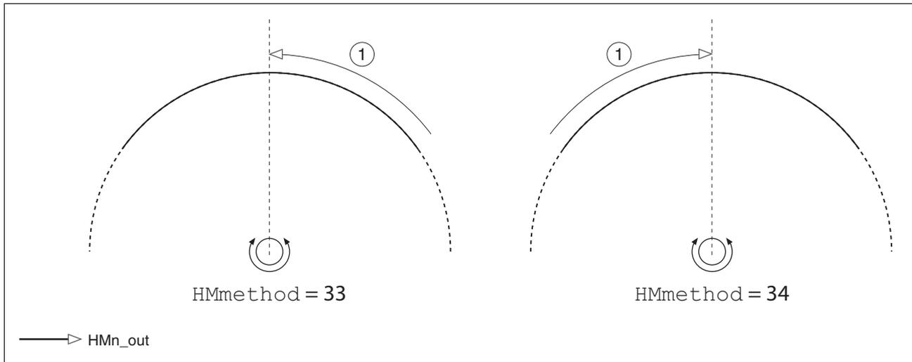
Figure 8.22 Reference movements to the index pulse
