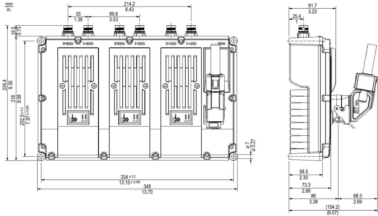
Figure 8-3: Dimensions of the Lexium 62 ILD (triple)
