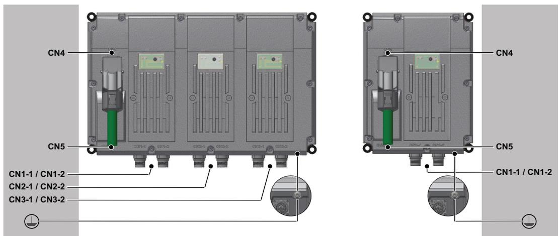
Figure 7-7: Connection overview Lexium 62 ILD Triple / Single Drive
