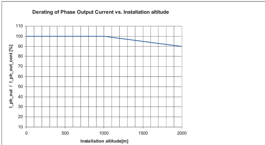
Figure 6-6: Power reduction at increased installation height (Lexium 62 ILD at 8 kHz clock frequency of power stage)
