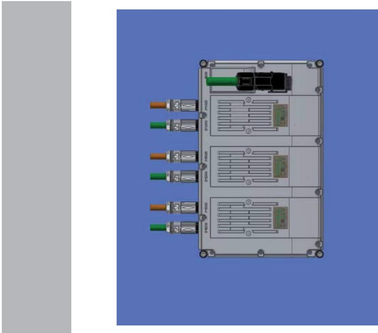
*Figure 7-3: Lexium 62 ILD mounting orientation vertical - cable leaving at left side*
