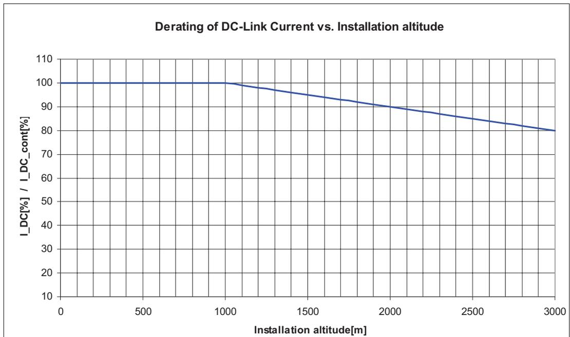
Figure 6-5: Power reduction at increased installation altitude (Lexium 62 connection module)
