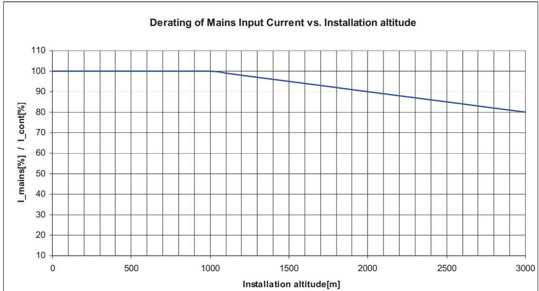
Figure 6-4: Power reduction at increased installation altitude (Lexium 62 power supply)
