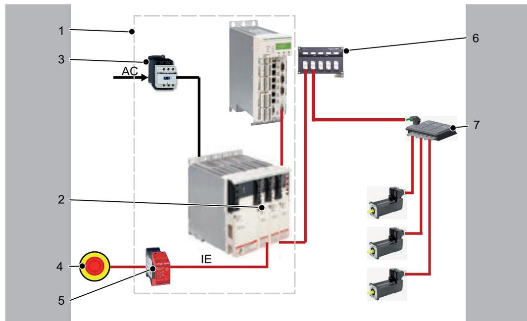
Figure 6-1: Lexium 62 drive system with emergency stop
