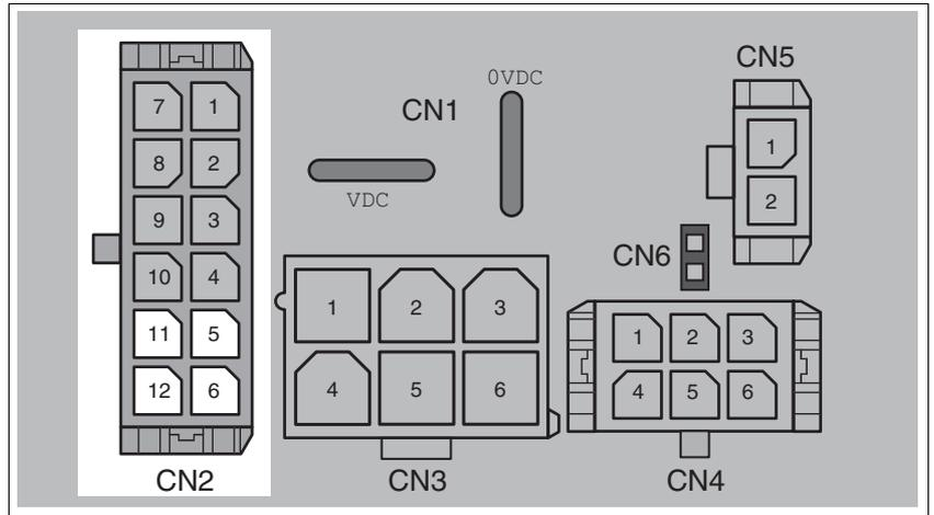
Figure 6.10 Pin assignment of Profibus fieldbus interface
