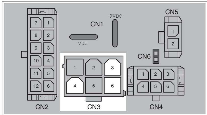
Figure 6.13 Pin assignment of CAN fieldbus interface
