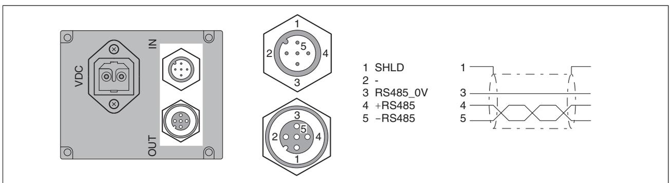
Figure 6.17 Pin assignment of the RS485 fieldbus interface
