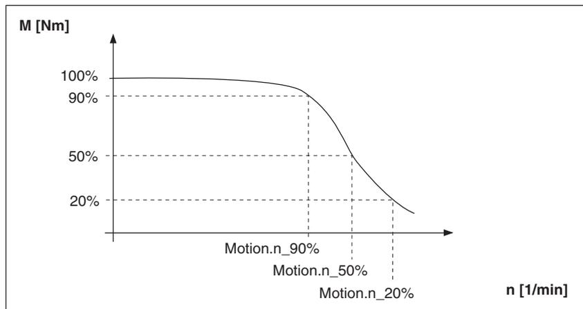
Figure 7.1 Typical torque characteristic of a stepper motor
