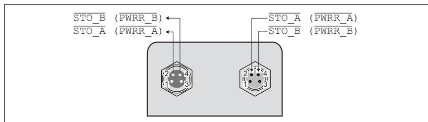
Figure 6.22 Pin assignment
