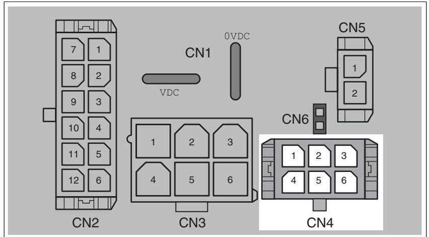
Figure 6.18 Pin assignment of the 24V signal interface
