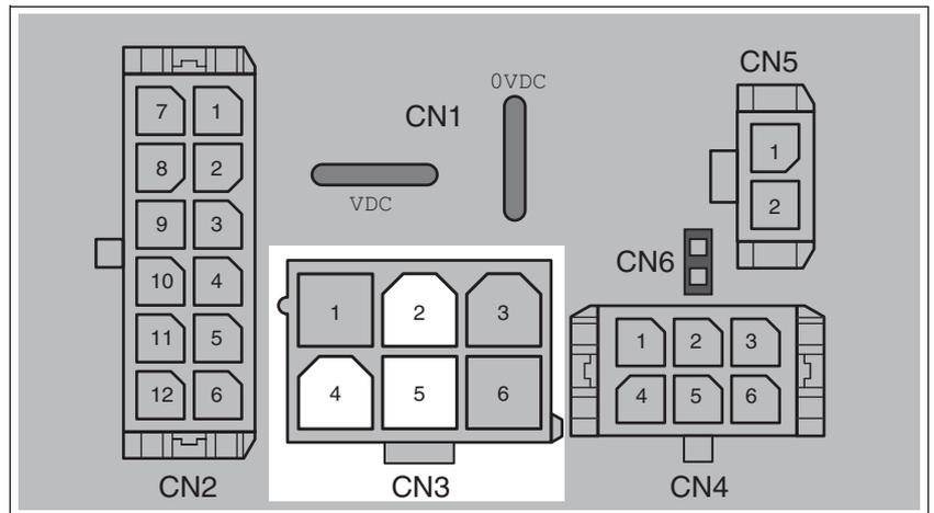
Figure 6.16 Pin assignment RS485
