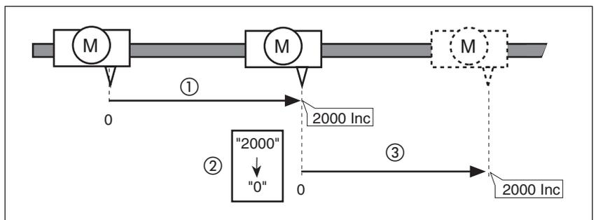
Figure 8.7 Positioning by 4000 increments with position setting
