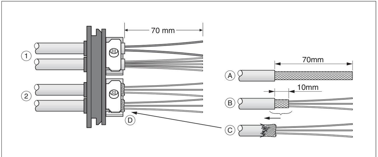
Figure 6.3 Fastening the cable in the cable entry
