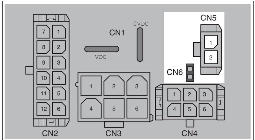
Figure 6.19 Pin assignment of safety function
