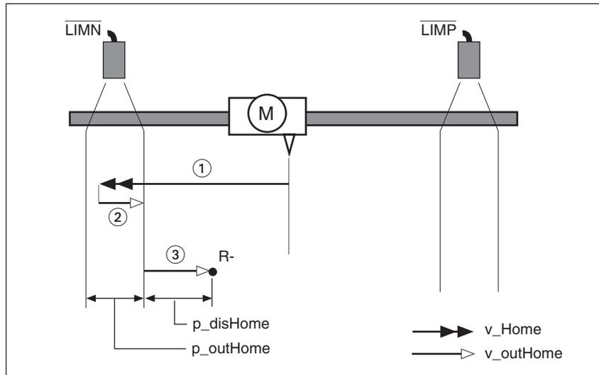
Figure 8.4 Reference movement to the negative limit switch
