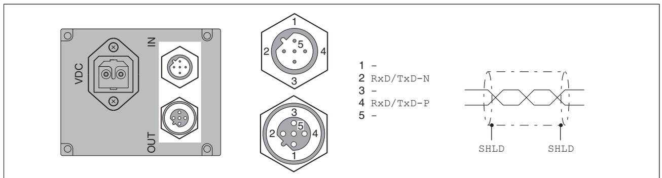
Figure 6.11 Pin assignment of Profibus fieldbus interface
