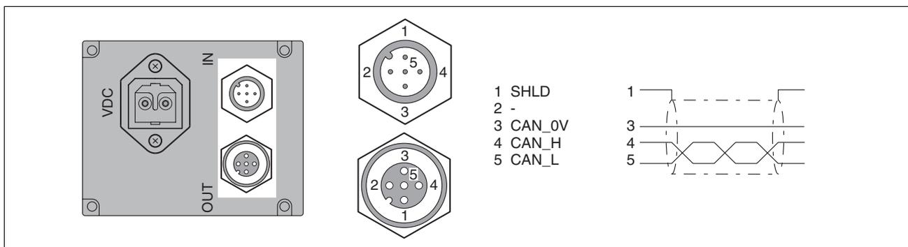
Figure 6.14 Pin assignment of CAN fieldbus interface
