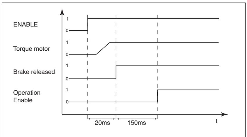
Figure 8.8 Releasing the holding brake
