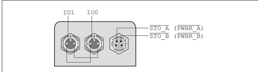
Figure 6.21 Pin assignment
