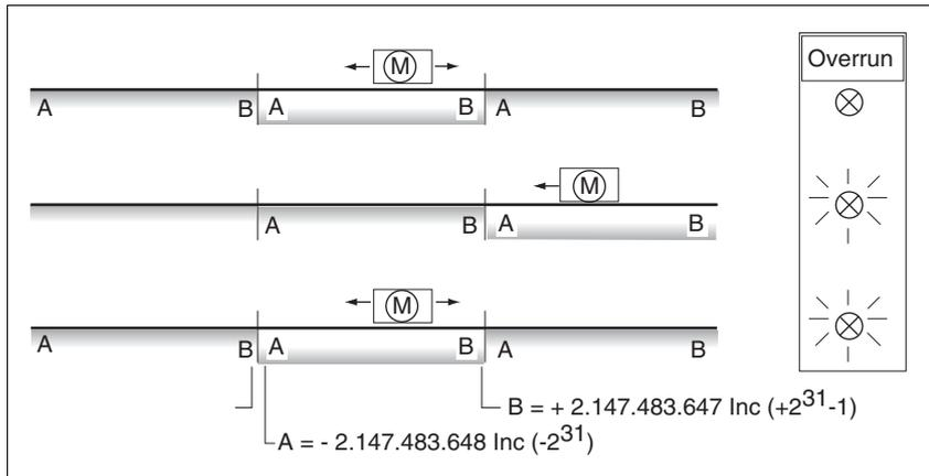
Figure 8.1 Positioning range and range overrun
