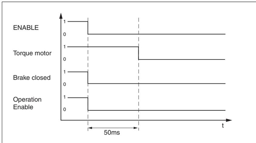
Figure 8.9 Applying the holding brake
