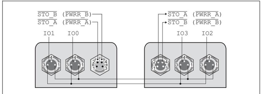
Figure 6.23 Pin assignment
