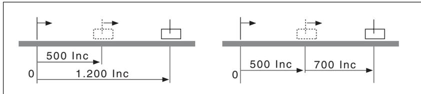
Figure 8.3 Absolute positioning (left) and relative positioning (right)
