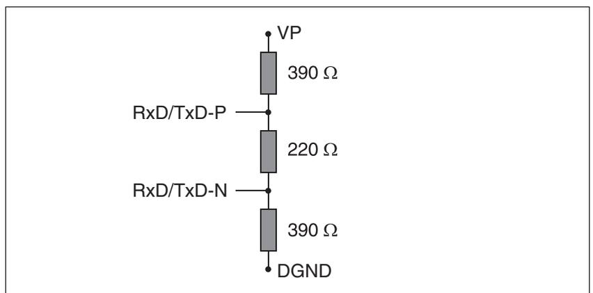
Figure 6.8 Terminating resistor
