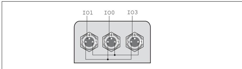
Figure 6.20 Pin assignment
