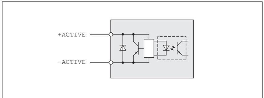
Figure 6.10 Signal output circuits with galvanic isolation
