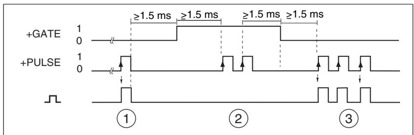
Figure 8.4 Signal sequences during switch-on via **GATE**
