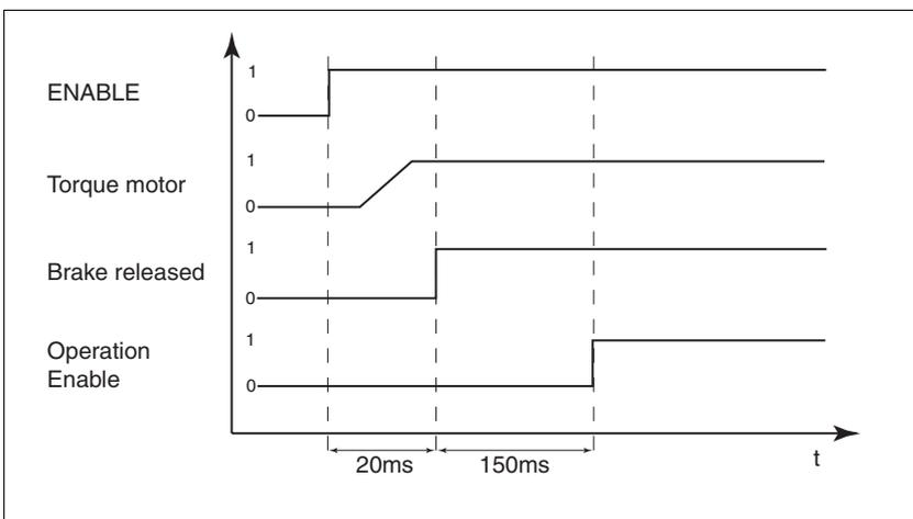
Figure 8.6 Releasing the holding brake
