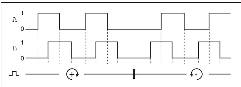
Figure 8.3 AB encoder signals
