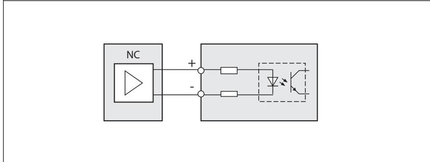
Figure 6.8 Signal input circuits with galvanic isolation
