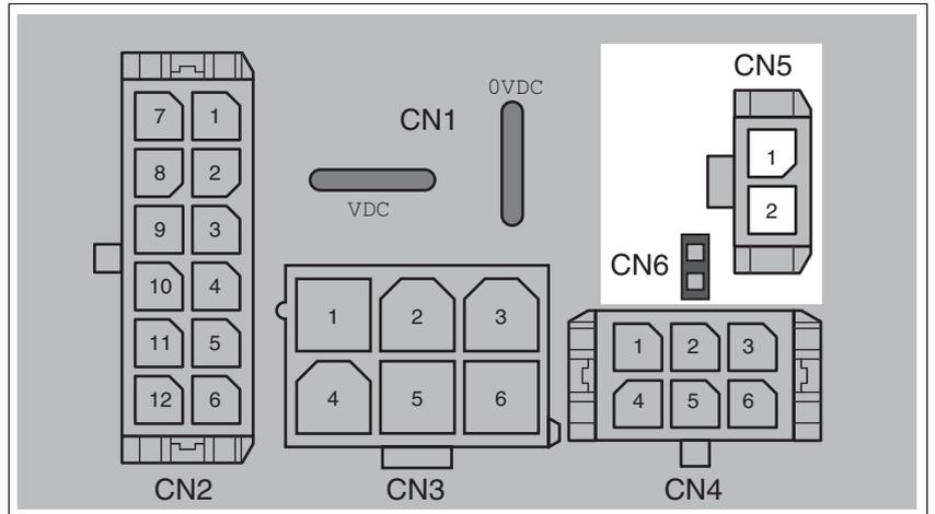
Figure 6.13 Pin assignment of safety function
