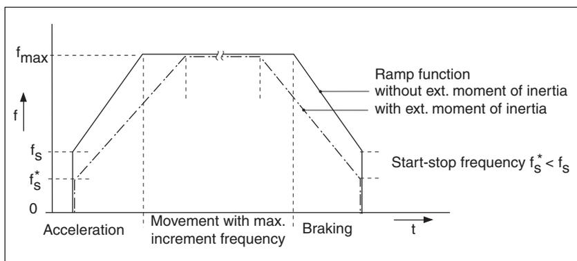
Figure 7.2 Characteristic curves of the linear ramp
