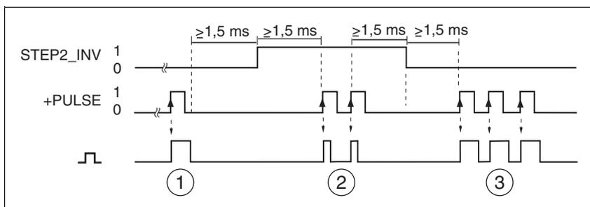
Figure 8.5 Signal sequences when the STEP2\_INV changes
