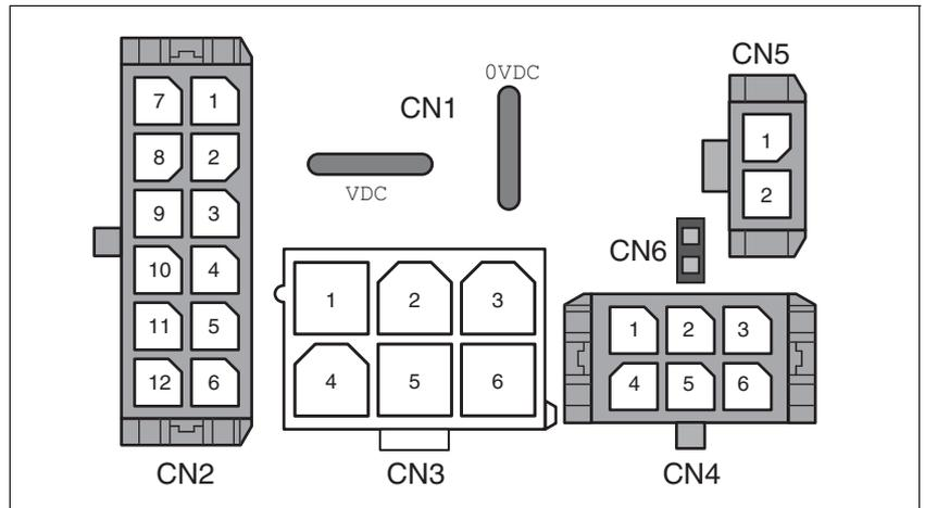
Figure 3.4 Overview of printed circuit board connectors
