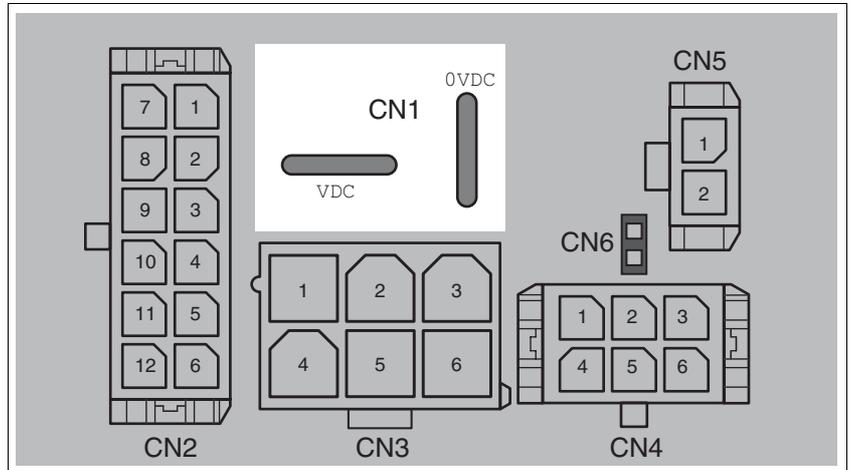
Figure 6.7 Pin assignment supply voltage
