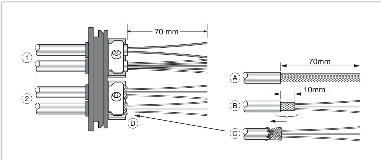
Figure 6.4 Fastening the cable in the cable entry
