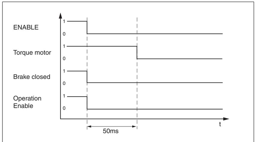
Figure 8.7 Applying the holding brake
