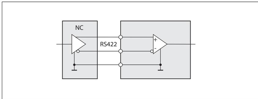
Figure 6.9 Signal input circuits without galvanic isolation
