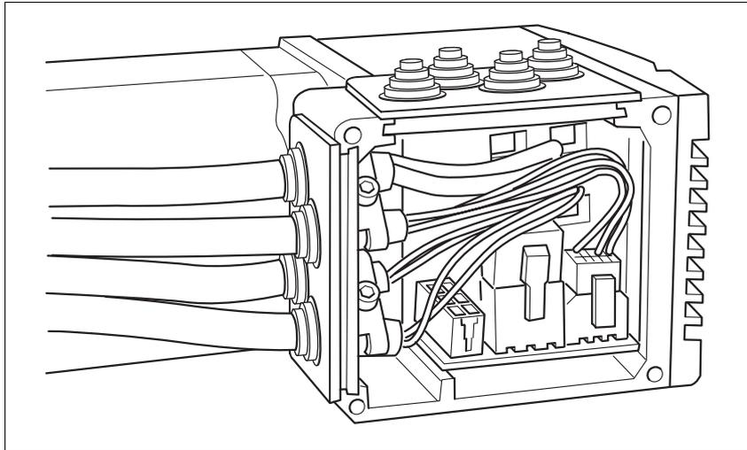
Figure 6.6 Inserting the cable entries
