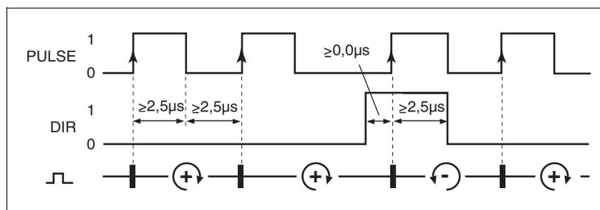
Figure 7.1 Checking the direction of rotation of the motor
