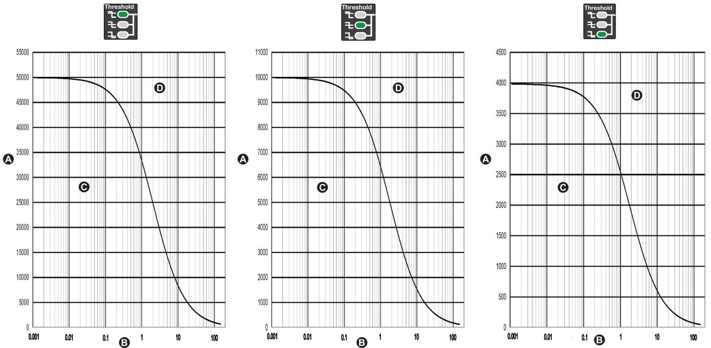
**en** Resistance vs system capacitance graph for the device threshold values.
