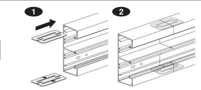
Installation of joint cover-piece kit
