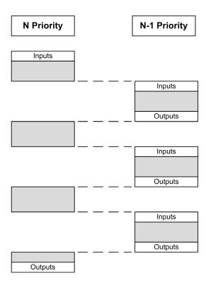
**NOTE:** If the same input is used in different tasks the input image may change during the task cycle of the lower priority task.
