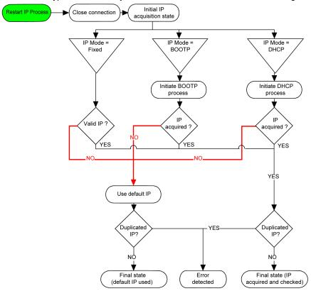
**NOTE:** If a device programmed to use the DHCP or BOOTP addressing methods is unable to contact its respective server, the controller uses the default IP address. It will, however, constantly repeat its request.
