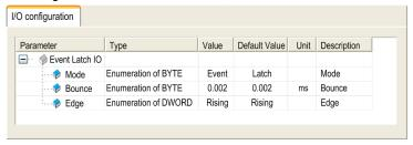
Event\_Latch inputs are used to enable event I/O or latched I/O and they are simple function added under **DM72F0** or **DM72F1** for input 0 to 3.
