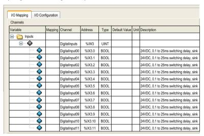
For further generic descriptions, refer to I/O Mapping Tab Description (see page 113). The table below describes the DI12DE I/O Mapping configuration:
