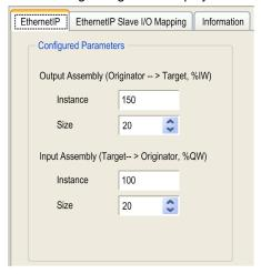
The EtherNet/IP configuration parameters are defined as:
