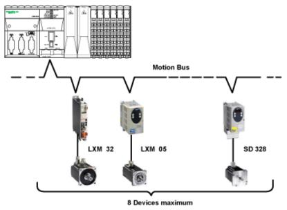
**NOTE:** In many cases, a daisy-chain network topology that does not use any tap-offs will provide improved performance. If you use a different topology and tap-offs to connect the motion devices on your CANmotion bus, these alternate topologies can exceed the capabilities of the CANmotion bus to provide synchronized motion control. It is essential to conduct thorough testing and commissioning before placing your CANmotion bus into service.
