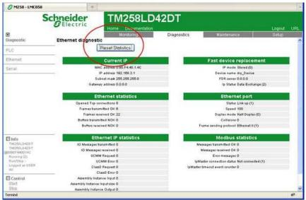
The **Reset Statistic** button sets the **Ethernet statistics** to 0.
