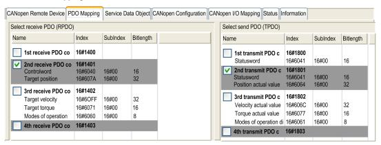
The default **PDO mapping** configuration of CANmotion slave is suitable for most implementations of the Cyclic Synchronous Position (CSP). If cyclic synchronous torque mode, cyclic synchronous velocity mode or optional TPDO are needed the PDO mapping has to be modified as follows:
