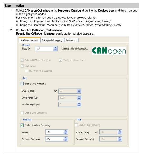
NOTE: If Enable Sync Producing is checked, the CANx\_Sync task is added.
