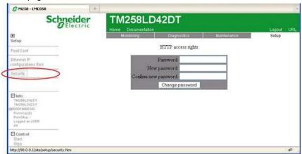
The password is case-sensitive and can be a mix of up to 10 alphanumerical characters (a...Z, 0...9).
