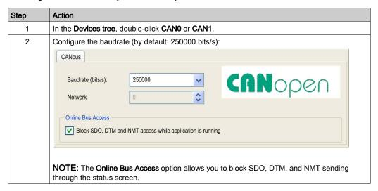
When connecting a DTM to a device using the network, the DTM communicates in parallel with the running application. The overall performance of the system is impacted and may overload the network, and therefore have consequences for the coherency of data across devices under control.
