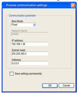
You can configure the Ethernet settings in the Process communication settings window in 2 ways:
