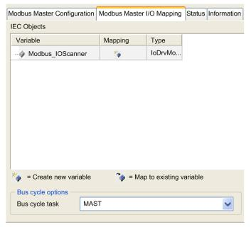
The Bus cycle task parameter allows you to select the application task that manages the scanner:
