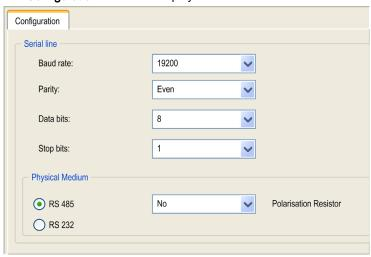
The following parameters must be identical for each serial device connected to the port.
