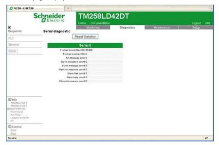
The **Reset Statistics** button sets the statistics of the serial connections to 0.
