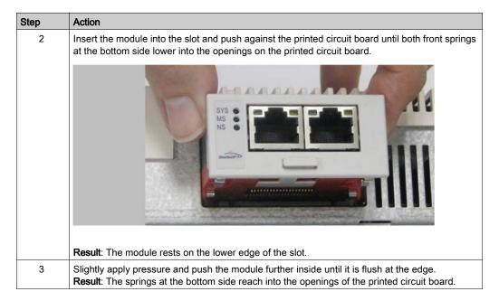
**NOTE:** Ensure that the module is flush at the edge.
