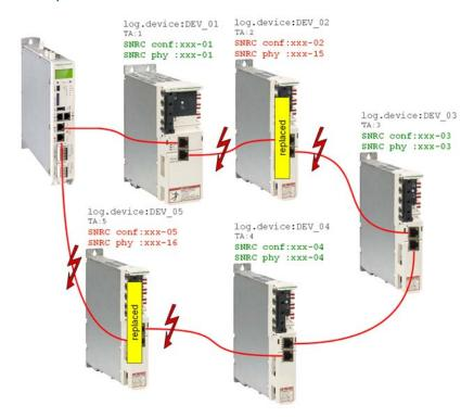
After the physical replacement of the devices the machine has to be restarted again. In order for the controller interface for FDR to be started, the parameter FDRStartMode has to be set to Start/1 or Phase start-up/2 and the parameter FDRConfirmationMode to by display / 0.
