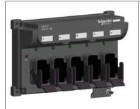
The Lexium 62 Distribution Box is the link between Lexium 62 Connection Module and Lexium 62 ILM. Depending on the number of drives, 1 to 4 Lexium 62 ILMs or daisy chain lines can be connected. When operating more than four drives, simply expand the system using one or more Lexium 62 Distribution Box.
