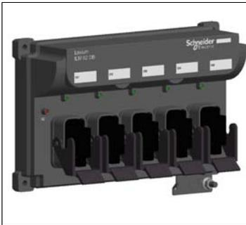
The Lexium 62 Distribution Box is the link between Lexium 62 Connection Module and Lexium 62 ILM. Depending on the number of drives, 1 to 4 Lexium 62 ILMs or daisy chain lines can be connected. When operating more than four drives, simply expand the system using one or more Lexium 62 Distribution Box.
