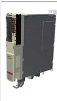
The Lexium 62 Connection Module supplies the Lexium 62 ILMs with DC voltage from the DC bus via a hybrid cable or via a power cable (daisy chain wiring). Additionally, the Lexium 62 Connection Module provides the Inverter Enable and Sercos interface.
