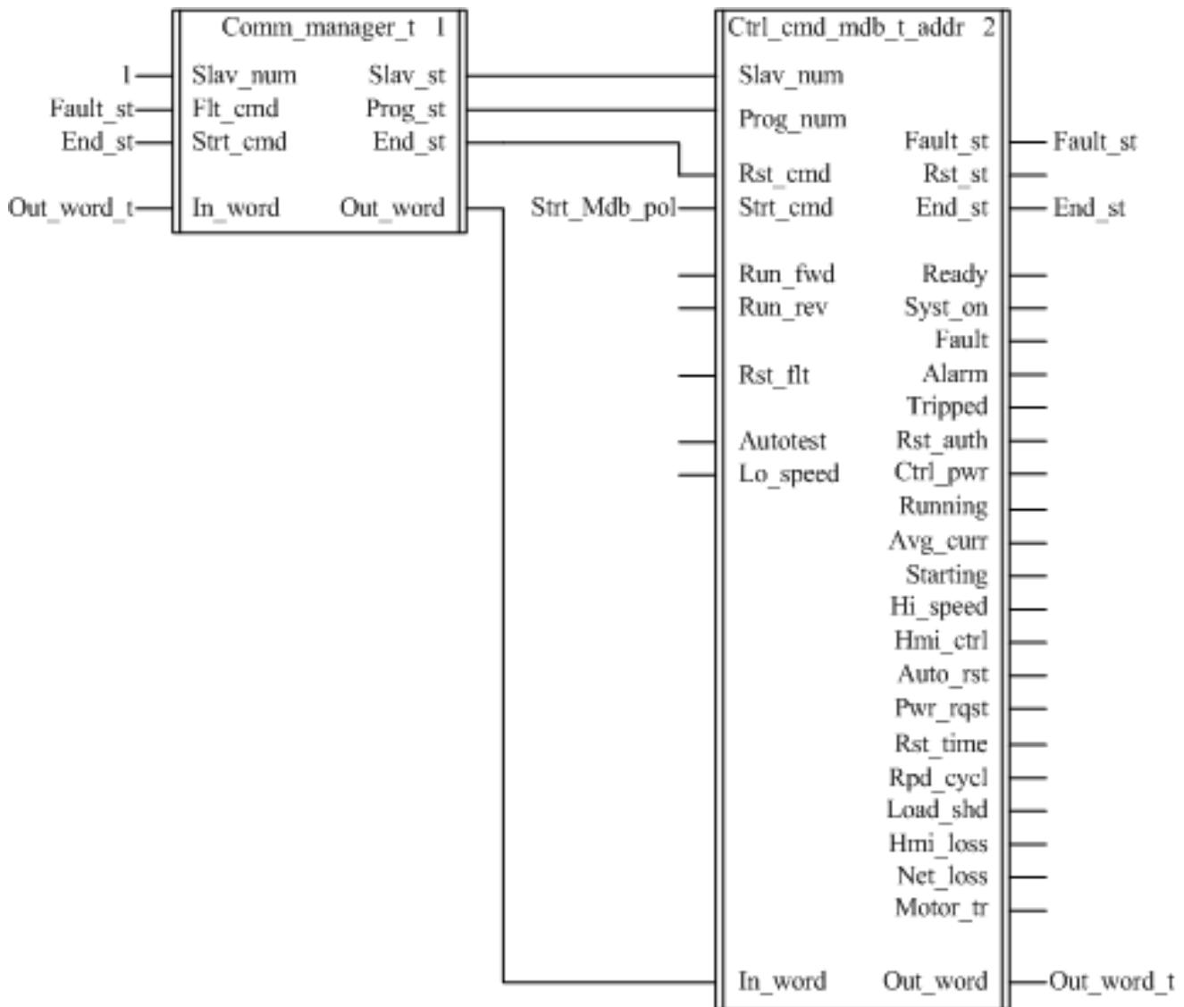
The Comm\_manager\_t DFB can be used in case both TeSys U starter-controllers and TeSys T motor management systems are present on the same Modbus SL network.
