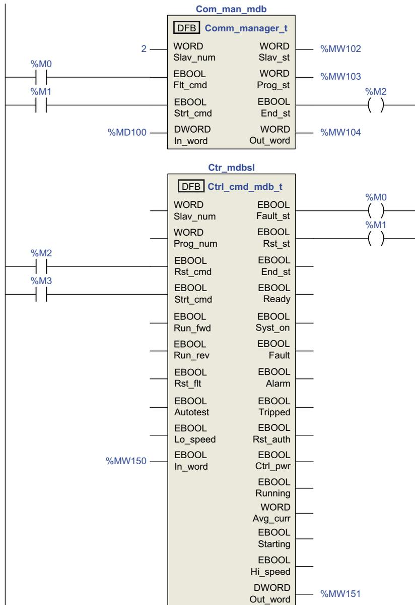
The Comm\_manager\_t DFB can be used in case both TeSys U starter-controllers and TeSys T motor management systems are present on the same Modbus SL network.
