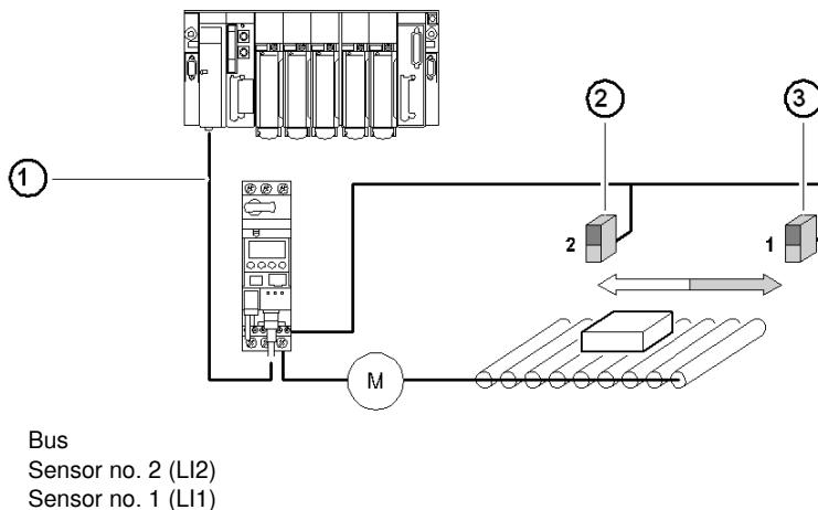
**NOTE:** In the case of a reversing starter, the reflex stop works in both directions. Sensor no. 2 (logic input LI2) has no effect on reflex operation.
