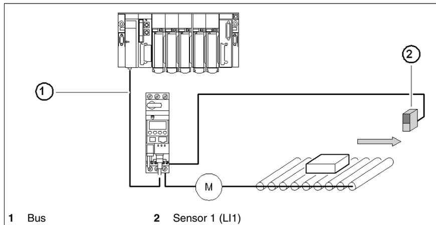
**NOTE:** In case of a reversing starter, reflex stop impacts both directions.
