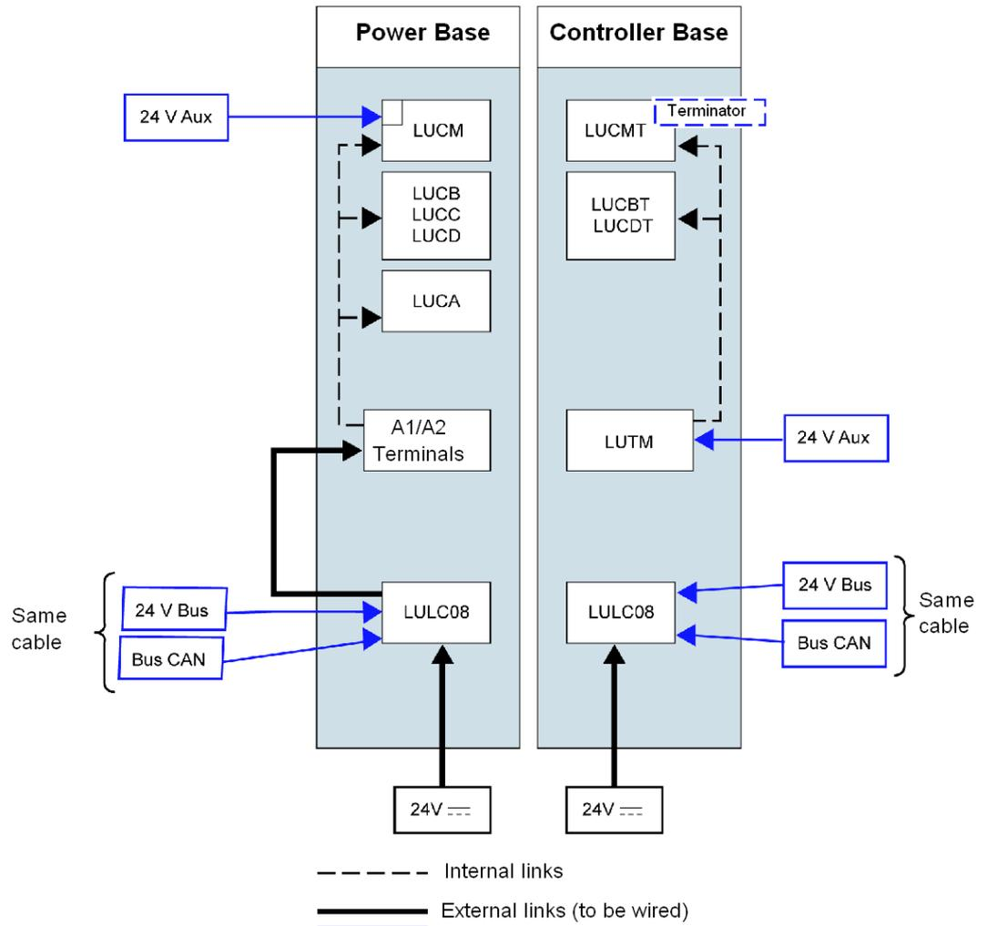
24V Bus = Communication module power supply (CAN\_V+ and CAN\_GND)
