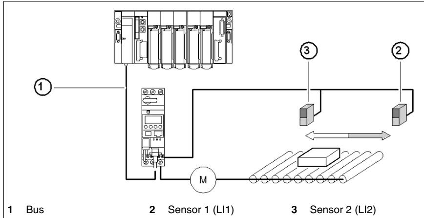
**NOTE:** Sensor 2 (LI2) does not impact the forward direction, and sensor 1 (LI1) does not impact the reverse direction.
