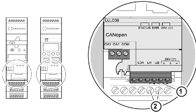
1. 24V  $\overline{---}$  power supply terminal for outputs OA1, OA3 and LO1 (if required)
