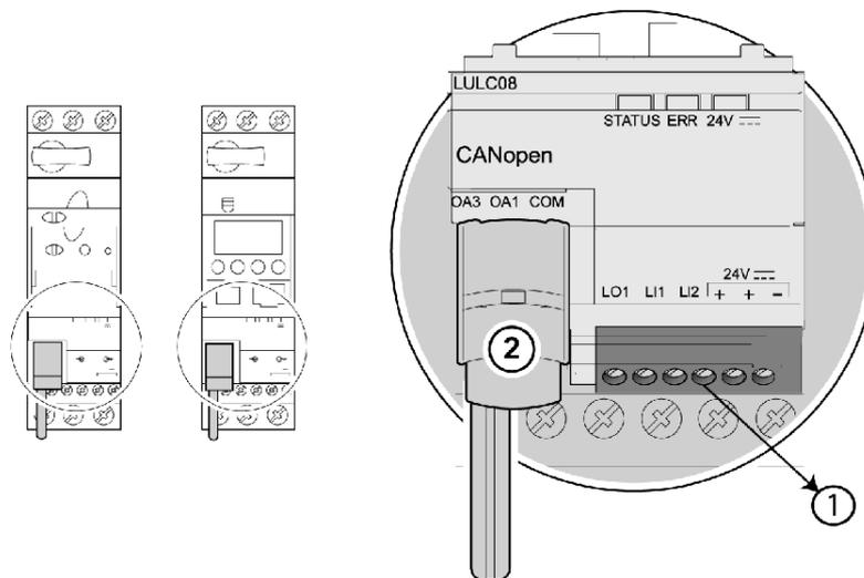
1. 24V  $\overline{\text{---}}$  power supply terminal for outputs OA1, OA3 and LO1
