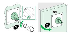
It is possible to temporarily disable this lock to open the door when the device is in the I (ON) position.
