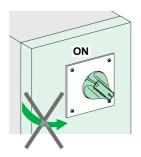
Locks the door in the closed position when the device is in the I (ON) position or in the Trip position.
