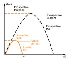
The exceptional limiting capacity of TeSys GV5 / GV6 devices is due to the rotating double-break technique (very rapid natural repulsion of contacts and the appearance of two arc voltages in-series with a very steep wave front).
