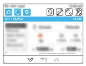
In the Device view, the device with its ERMS mode engaged displays an ERMS message in the title bar.
