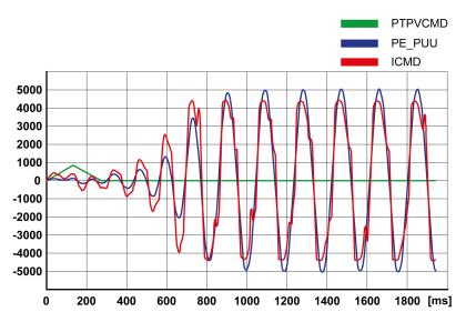
**NOTE:** The process of tuning requires trials of successive approximations. Values that are too high or too low relative to the other relevant values might cause instability. If it is necessary to have a low or high value of the parameter in the preceding example, you may need to adjust the values of the other relevant parameters to compensate and achieve a stable system.
