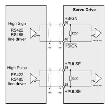
Connect the cable shield to the equipotential ground of your controller/drive electrical system.
