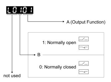
The following table provides an overview of the possible signal output functions:
