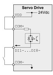
Example of digital input (negative logic) with external power supply:
