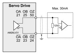
Example of encoder output signal, high-speed optocoupler.
