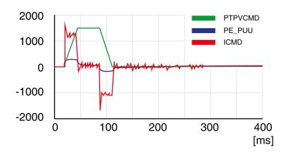
Example P8-03 (LTNP) value too high - oscillation at standstill (65 Hz)
