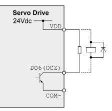
Example of digital output DO6 (OCZ) with external power supply (negative logic):
