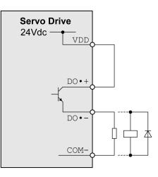
Example of digital outputs DO1 ... DO5 with external power supply (positive logic):
