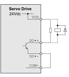
Example of digital outputs DO1 ... DO5 with external power supply (negative logic):
