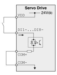
Example of digital input with external power supply (positive logic):
