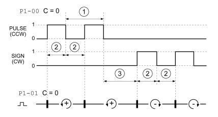
The signal shape shown relates to the factory setting (P1-00 C=0). The direction of movement shown relates to the factory setting (P1-01 C=0).
