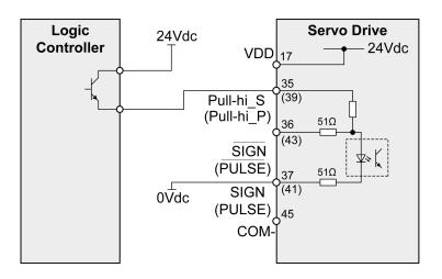
Example of pulse input (open collector) with external power supply (positive logic).
