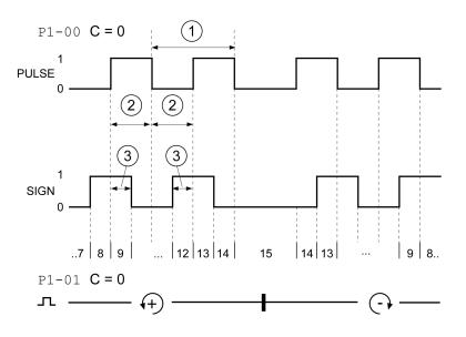
The signal shape shown relates to the factory setting (P1-00 C=0). The direction of movement shown relates to the factory setting (P1-01 C=0).
