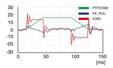
Example P8-20 (NLPEAFF) negative position deviation during acceleration phase (100 Hz)
