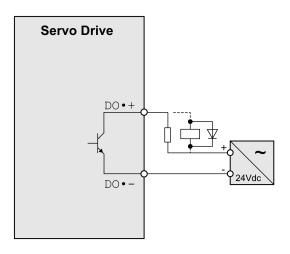
Example of digital output DO6 (OCZ) with internal power supply (negative logic):
