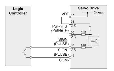
Example of pulse input (open collector) with external power supply (negative logic).
