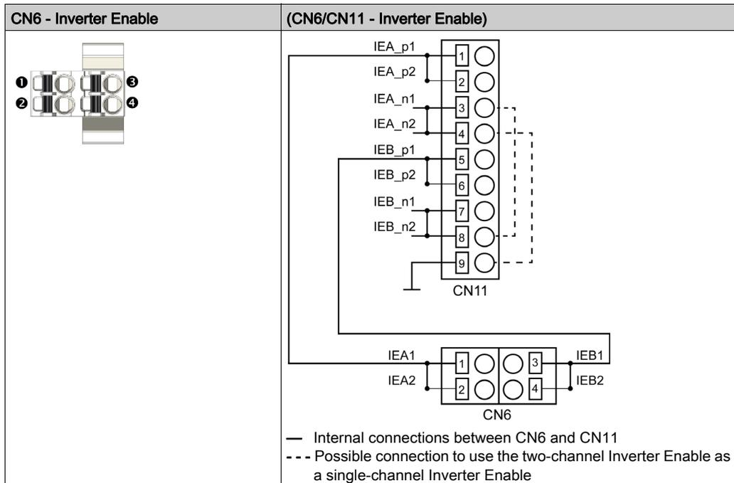
Electrical connection - Inverter Enable
