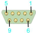
Electrical connection D-Sub 9-pin male connector
