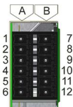
Electrical connection - digital inputs / outputs
