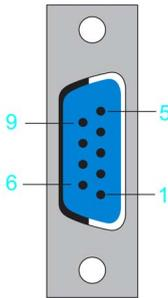
Electrical connection D-Sub 9-pin female connector
