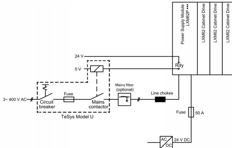
**NOTE:** The 24 Vdc supply input current must be limited to 50 A, which can be realized by a 50 A fuse as shown above. In particular, a 50 A fuse is mandatory if a passive 24 Vdc power supply is used.
