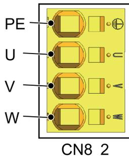
Electrical connection - motor connector
