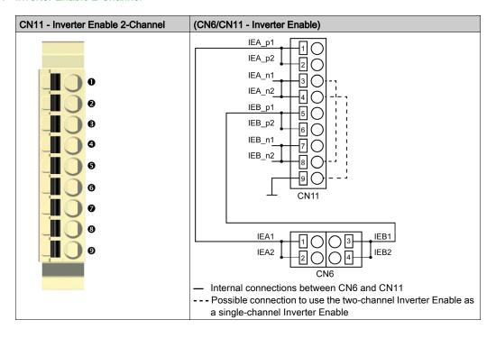
CN11 - Inverter enable 2-channel
