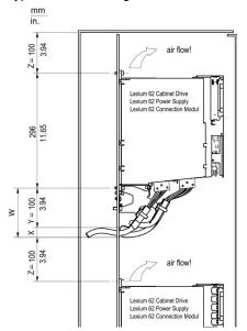
Type B: cable routing in cabinet behind mounting-backplane:
