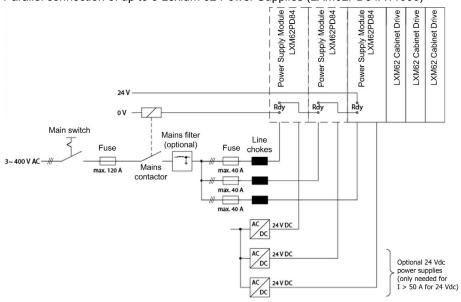
No fuses are required for the 24 Vdc supply inputs, if appropriate 24 Vdc power supply units are used which ensure that the output current remains below 50 A.
