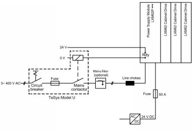
**NOTE:** The 24 Vdc supply input current must be limited to 50 A, which can be realized by a 50 A fuse as shown above. In particular, a 50 A fuse is mandatory if a passive 24 Vdc power supply is used.
