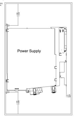
• Do not lay any cables or cable channels over the servo amplifiers or braking resistor modules.
