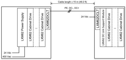
Topology 5: Coupling of More Than Two Control Cabinets in Line Topology
