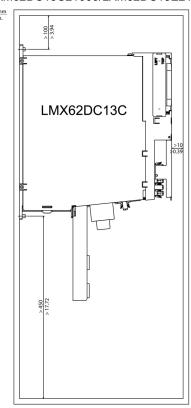
• Do not lay any cables or cable channels over the servo amplifiers or braking resistor modules.
