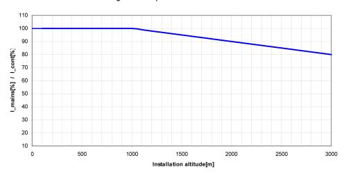
**NOTE:** Multiply the values with the nominal current at 40 °C (104 °F) in order to calculate the maximum continous current value, depending on the required installation altitude.
