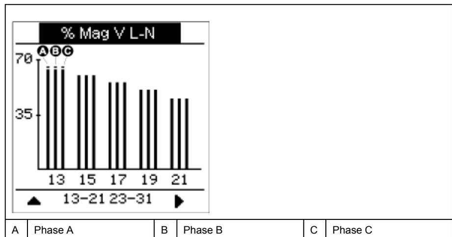
The vertical axis of the harmonics graph indicates the harmonic's magnitude as a percentage of the fundamental harmonic, and is scaled based on the largest harmonic displayed. At the top of each vertical bar is a marker that shows the maximum value of the harmonic. If the harmonic is greater than the fundamental harmonic, this marker is triangular-shaped to show that the value is out of range.
