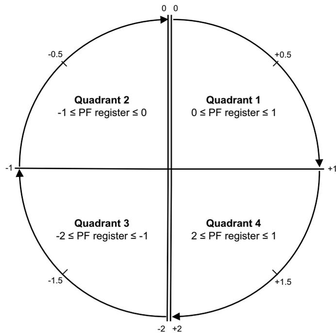
The PF value is calculated from the PF register value using the following formulas:
