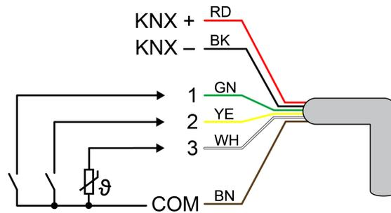
Image 2: Connection assignment of control cable (example)
