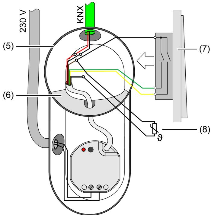
Image 3: Mounting example in electronic device box with partition wall, series push-button and NTC temperature sensor
