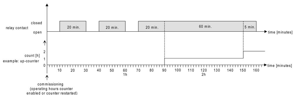
Image 11: Function of the operating hours counter (using the example of counted hours)
