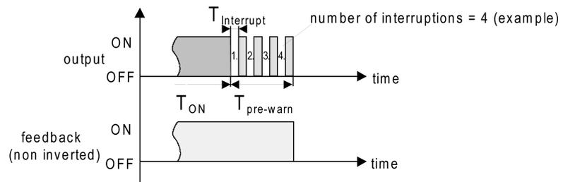
Image 8: The pre-warning function of the staircase function (example)
