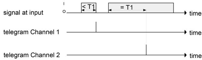
Image 24: Example of operation concept "Channel 1 or Channel 2"
