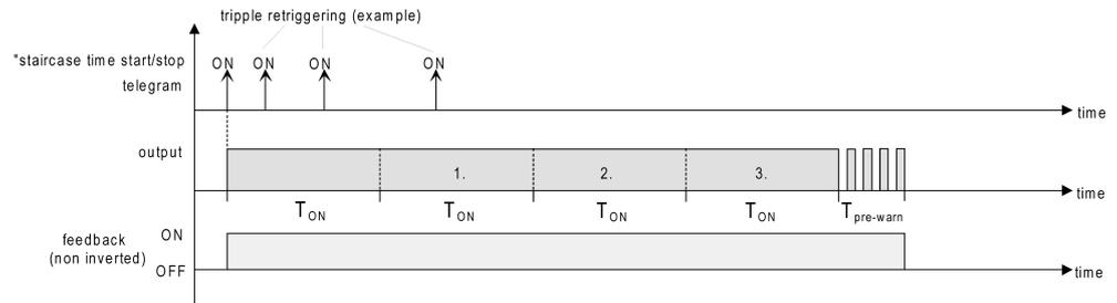
Image 9: Time extension of the staircase function
