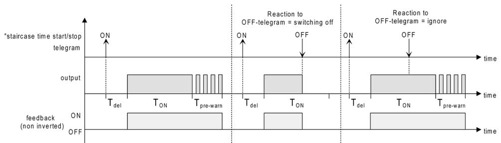
Image 7: Switch-off behaviour of the staircase function
