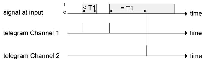
Image 25: Example for operation concept "Channel 1 and channel 2"
