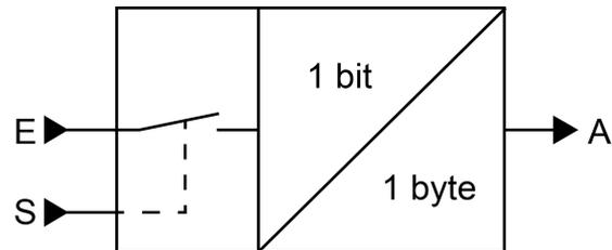
Image 26: Converter (1 bit -> 1 byte)
