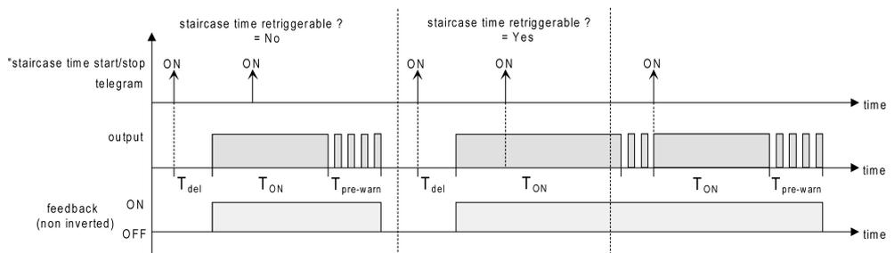
Image 6: Switch-on behaviour of the staircase function
