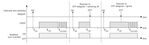
Image 25: Switch-off behaviour of the staircase function
