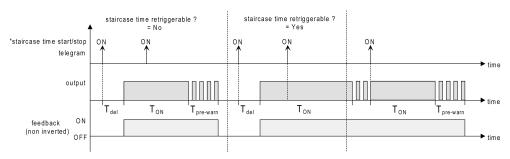
Image 24: Switch-on behaviour of the staircase function
