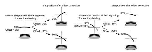
Image 18: Functional principle of slat offset (example showing slat type 1 / slat type 2 identical)
