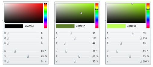
Image 43: Examples of brightness adjustment using the colour picker of the ETS Examples of HSV-RGB conversion:
