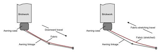
Image 21: Fabric stretching in an awning
