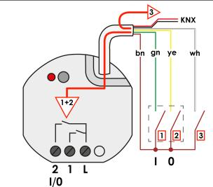
Image 33: Functionality of the inputs when controlling the internal switching output 2 as two-area operation
