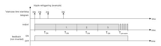
Image 27: Time extension of the staircase function
