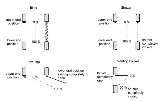
Image 9: Positions defined as a function of the type of movement
