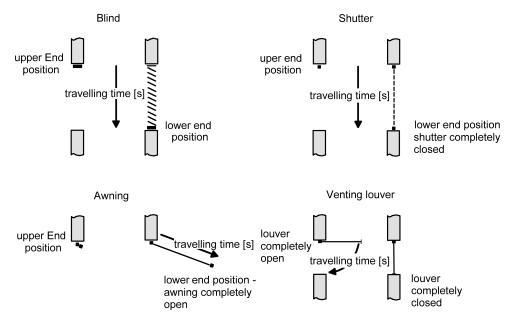
Image 6: Determining the movement time according to the drive type
