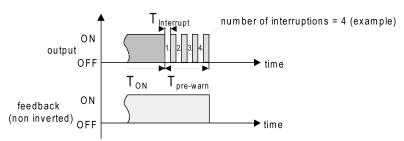
Image 26: The pre-warning function of the staircase function (example)
