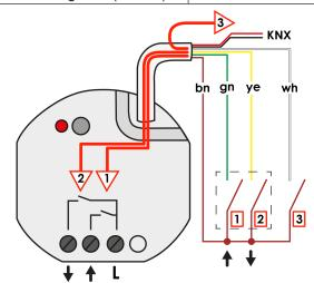
Image 30: Functioning of the inputs when controlling the the internal blind output
