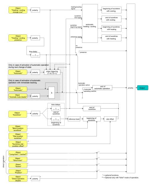
Image 20: Schematic function diagram of automatic heating/cooling
