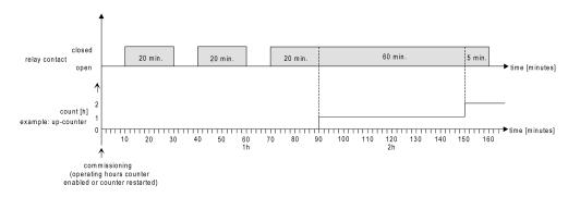
Image 29: Function of the operating hours counter (using the example of counted hours)
