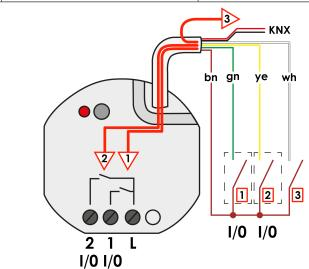
Image 31: Functionality of the inputs when controlling the internal
