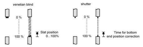
Image 22: End position correction of a Venetian blind or shutter
