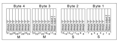
Image 23: Object structure of the collective feedback
