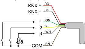
Image 2: Connection assignment of control cable (example)
