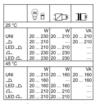
Image 7: Connected load conventional lamps
