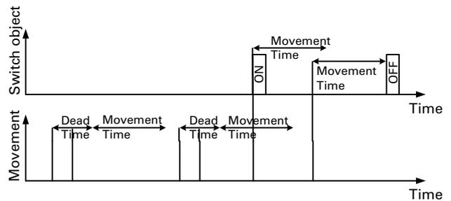
In master mode or normal mode the movement time corresponds to the staircase timer in the diagram above. In slave mode or monitoring mode the movement time corresponds to the cycle time. In practice a large number of applications can be implemented by means of the various blocks and sensors.
