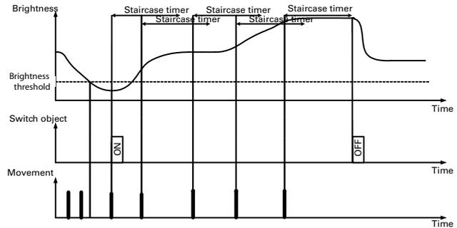
Where this differs from the presence detector is that the movement detector changes to non-brightness-dependent mode once the start of movement action (sending an ON telegram) has been carried out. Here freshly detected movements can retrigger the staircase timer. Unlike the presence detector, the movement detector cannot process the brightness jump and there is not even any setting of a hysteresis.
